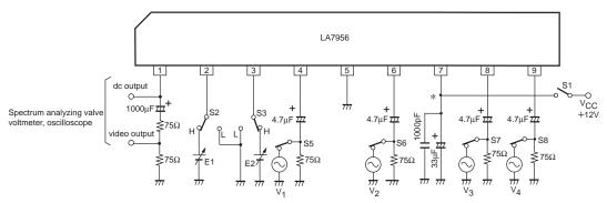
$\ast$  : Connect the bypass capacitor for  $V_{\mbox{CC}}$  as close to pin 7 as possible.
