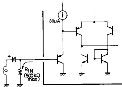
If a resistor of more than 500 k $\Omega$  is connected across input pin and GND, the noise (output) caused by amp 1 and amp 2 select is liable to increase at the time of F/R switching.
