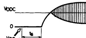
Example of rise waveform at pin 4 (or 17)
