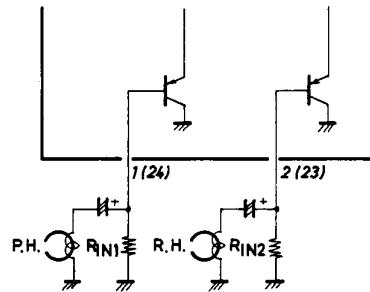
The difference in the value between  $R_{IN1}$  and  $R_{IN2}$  causes the variation in amp output DC voltage at the time of F/R switching. Therefore, the input DC voltage (voltage across  $R_{IN}$ ) must be made as equal as possible.
