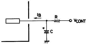
To turn ON the control circuit to finish the operation,  $I_B$  is required. Control voltage  $V_{OUT}$  is obtained with  $I_B$  of 4 μA min.
