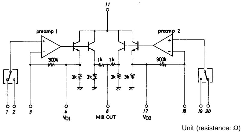
The MIX OUT output level  $V_O$  MIX at the time a signal is applied to preamp1 (or preamp2) only is 1/2 as compared with output levels  $V_{O1}$ ,  $V_{O2}$  at the time the same input signal is applied to both channels.
