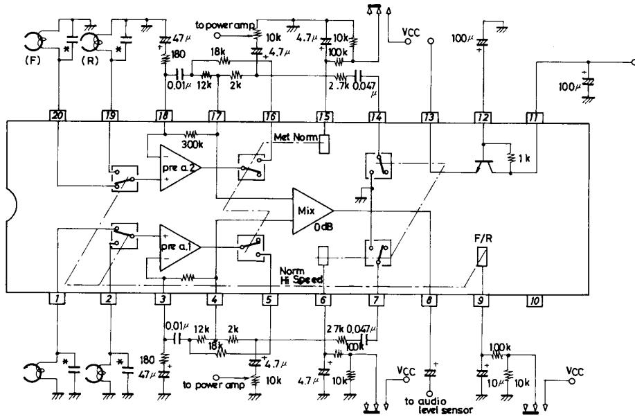
Unit (resistance: Ω, capacitance: F)
