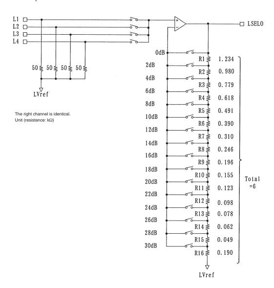
• Treble and bass band block internal equivalent circuit
