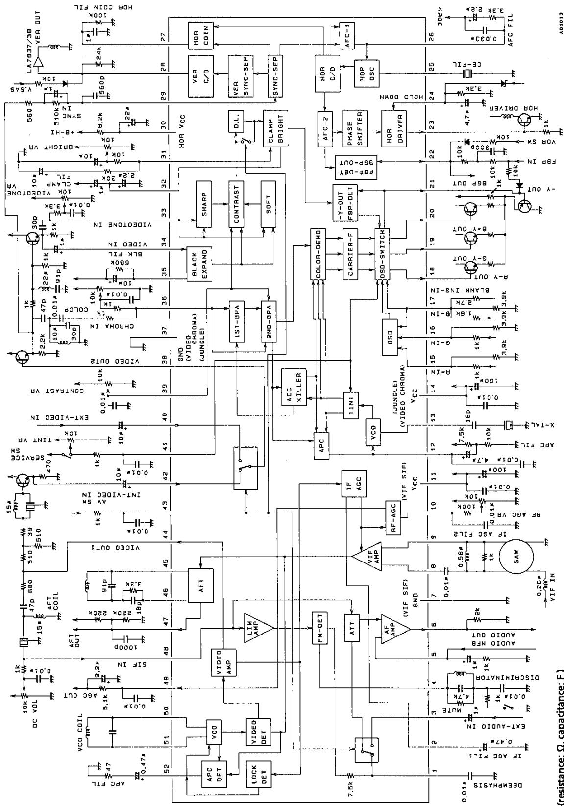
Unit (resistance:  $\Omega$ , capacitance: F)
