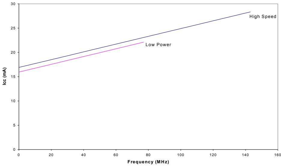
The typical pattern is a 16-bit up counter, per logic block, with outputs disabled.
