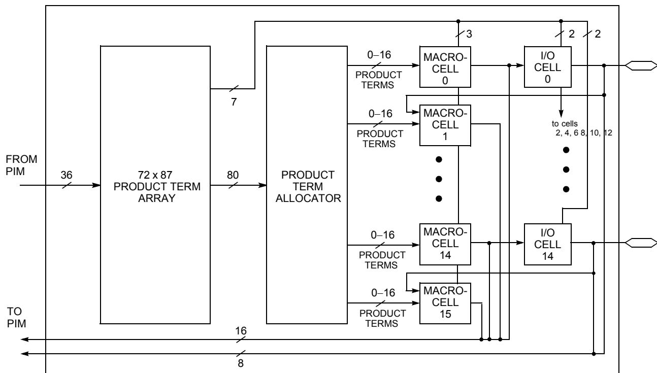
**Figure 1. Logic Block with 50% Buried Macrocells**
