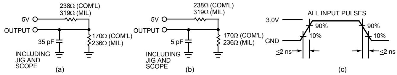
**3.3V AC Test Loads and Waveforms**
