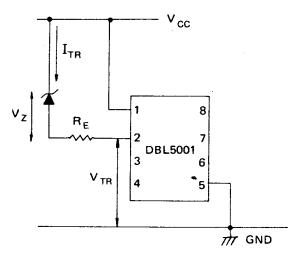
To operate the 5001 circuit from a DC 12V supply, R<sub>E</sub> should be typically  $50 \text{K}\Omega$ . This operation can also be used to reduce the effective value of the V  $_{\text{CC(INI)}}$ , by inserting a zener diode in series with R<sub>E</sub>. Then, this initiating voltage V  $_{\text{CC(INI)}}$  is V  $_{\text{IR}} + \text{V}_{\text{Z}} + 10 \text{R}_{\text{E}}$ .
