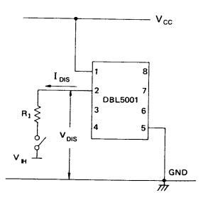
When the 5001 circuit is oscillating, this circuit may be inhibited for voltage in the range  $V_{CC(INI)} < V_{CC} \le V_{CC(MAX.)}$  by sinking the current from  $D_1$ , starving  $Q_1$  of base current. This is achieved by either grounding pin 2 or applying a voltage  $V_{IH}$  via a resistor  $R_1$  to pin 2.
