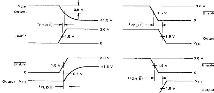
H = High-Logic State, L = Low-Logic State, Z = High Impedance State
