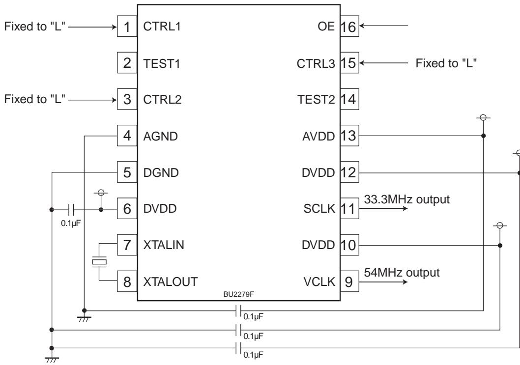
Remarks) The IC is basically needed to be on the board. (Unless it is on the board, the characteristics are not guaranteed.) Decoupling capacitance(0.1µF) is needed to be placed between 13PIN(AVDD) and 4PIN(AGND).Decoupling capacitance(0.1µF)is needed to be placed between 16PIN(DVDD) 10PIN(DVDD), 12PIN(DVDD) and 5PIN(DGND) each.
