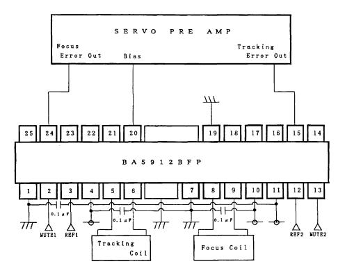
When used at Pre Vcc > Pow Vcc + VF and in the standby mode, REF1 (PIN3) and REF2 (PIN12) must be set to open, or 0.5V or less. When used with REF1 (PIN3) and REF2 (PIN12) shorted; or MUTE1 (PIN2) and MUTE2 (PIN13) shorted, each microcomputer output must be able to supply a current of  $300\mu$ A or so.
