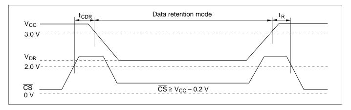
Low  $V_{CC}$  Data Retention Timing Waveform (2) ( $\overline{LB}$ ,  $\overline{UB}$  Controlled)
