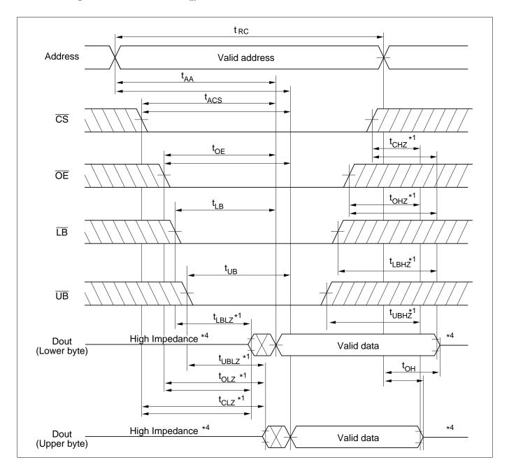
Read Timing Waveform (2)  $(\overline{WE}=V_{IH},\overline{LB}=V_{IL},\overline{UB},=V_{IL})$
