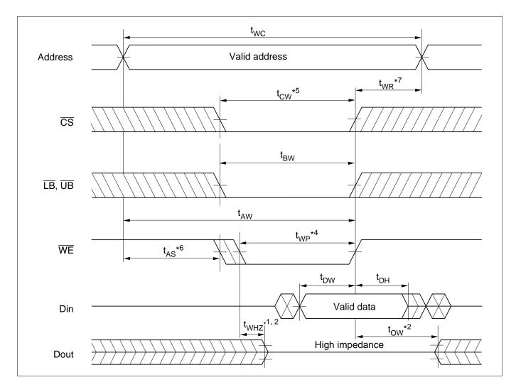
Write Cycle (2) ( $\overline{CS}$  Clock,  $\overline{OE} = V_{IH}$ )
