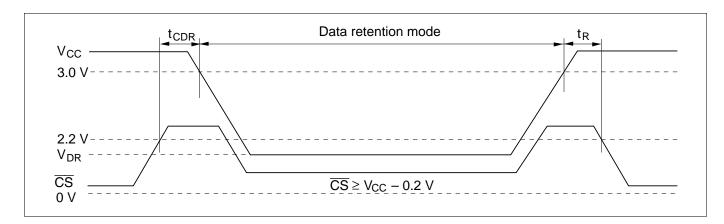
Low V<sub>CC</sub> Data Retention Timing Waveform (2) (LB, UB Controlled)
