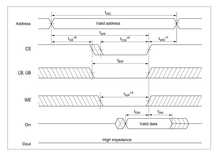
Write Cycle (3) ( $\overline{LB}$ ,  $\overline{UB}$  Clock,  $\overline{OE} = V_{IH}$ )
