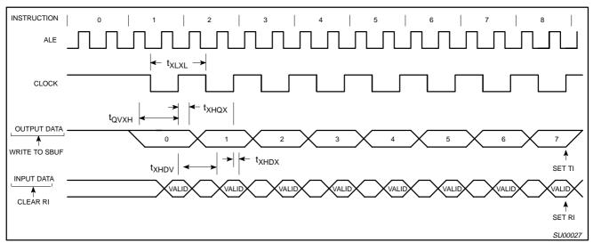
Figure 21. Shift Register Mode Timing
