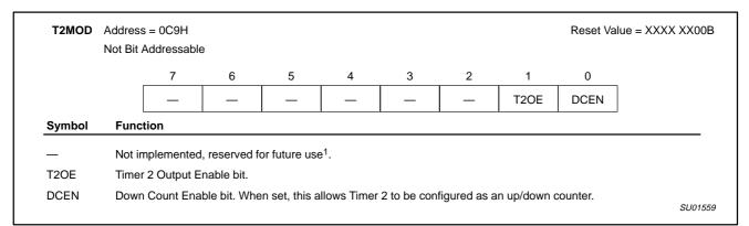
User software should not write 1s to reserved bits. These bits may be used in future 8051 family products to invoke new features. In that case, the reset or inactive value of the new bit will be 0, and its active value will be 1. The value read from a reserved bit is indeterminate.
