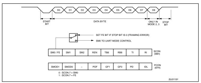
Figure 8. UART Framing Error Detection
