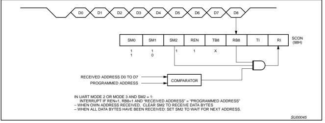
Figure 9. UART Multiprocessor Communication, Automatic Address Recognition
