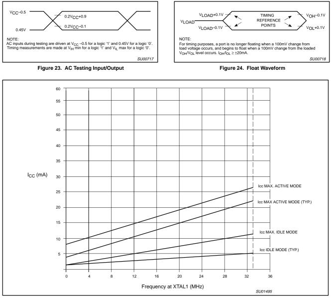
Figure 25. I<sub>CC</sub> vs. FREQ Valid only within frequency specifications of the device under test
