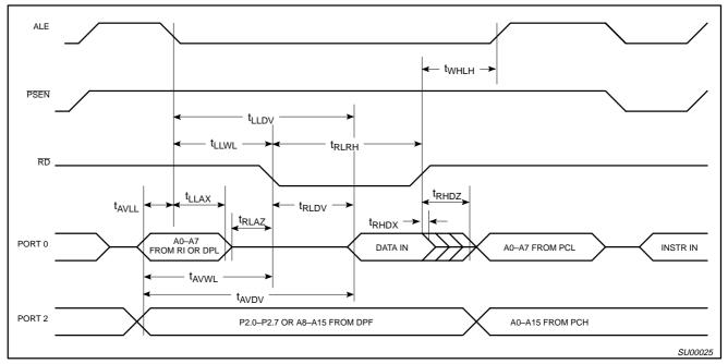
Figure 19. External Data Memory Read Cycle
