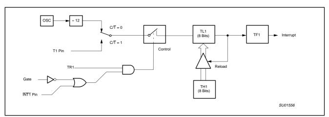
Figure 4. Timer/Counter 0/1 Mode 2: 8-Bit Auto-Load (Timer 1 shown)
