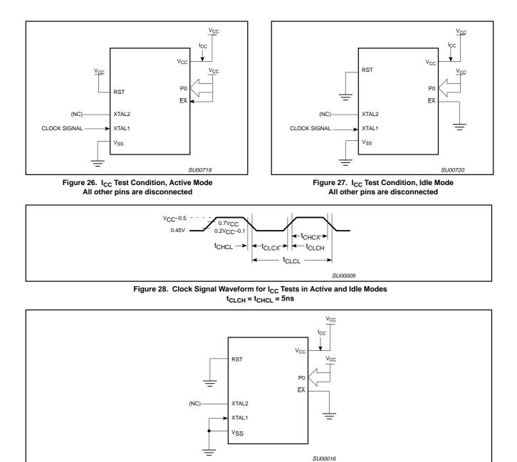
Figure 29. I<sub>CC</sub> Test Condition, Power Down Mode All other pins are disconnected.  $V_{CC}$  = 2V to 5.5V
