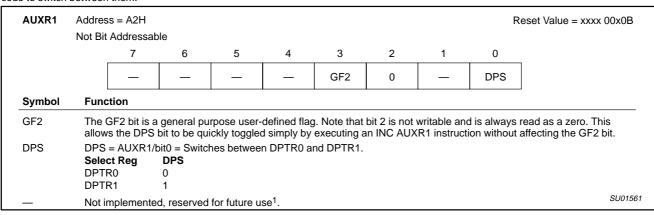
User software should not write 1s to reserved bits. These bits may be used in future 8051 family products to invoke new features. In that case, the reset or inactive value of the new bit will be 0, and its active value will be 1. The value read from a reserved bit is indeterminate.
