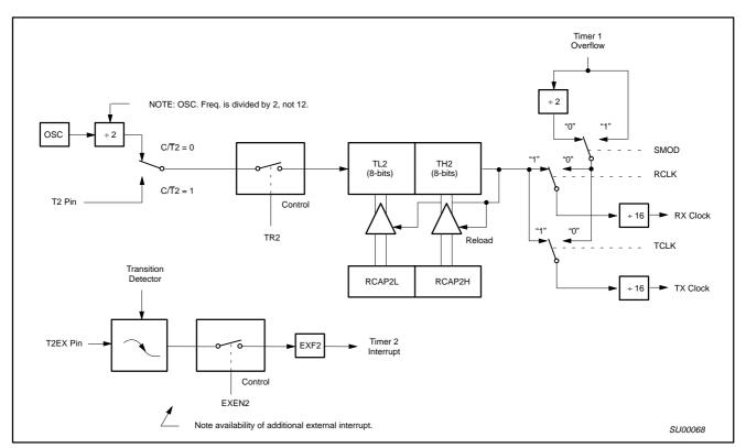
Figure 6. Timer 2 in Baud Rate Generator Mode
