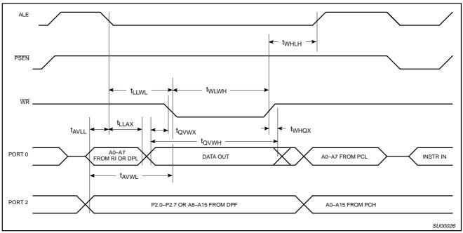
Figure 20. External Data Memory Write Cycle
