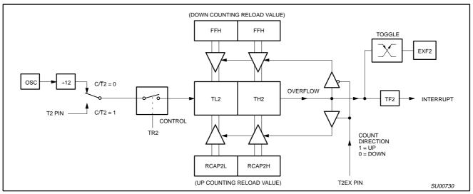
Figure 5. Timer 2 Auto Reload Mode (DCEN = 1)
