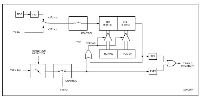
Figure 4. Timer 2 in Auto-Reload Mode (DCEN = 0)
