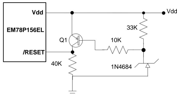
**Fig. 17 Circuit 1 for the Residue Voltage Protection**
