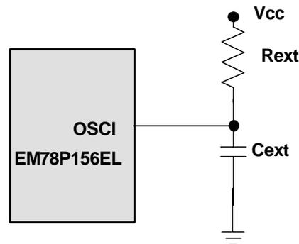
**Fig. 15 Circuit for External RC Oscillator Mode**
