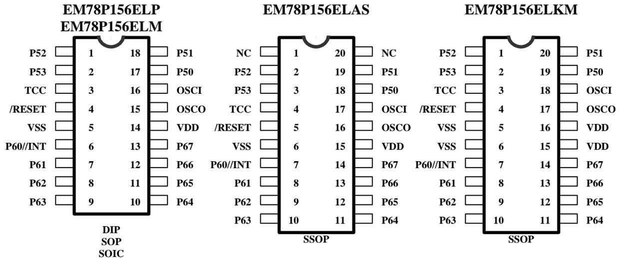
Fig. 1 Pin Assignment
