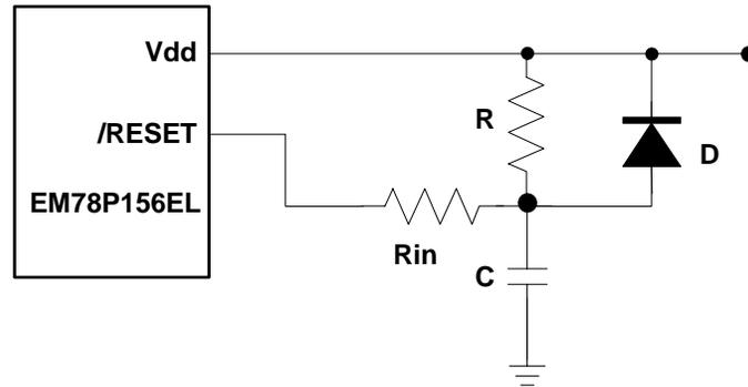
**Fig. 16 External Power-Up Reset Circuit**
