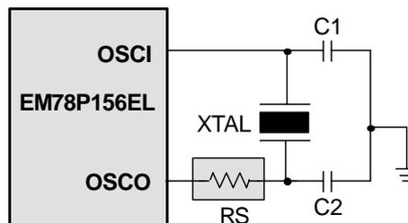
**Fig. 12 Circuit for Crystal/Resonator**
