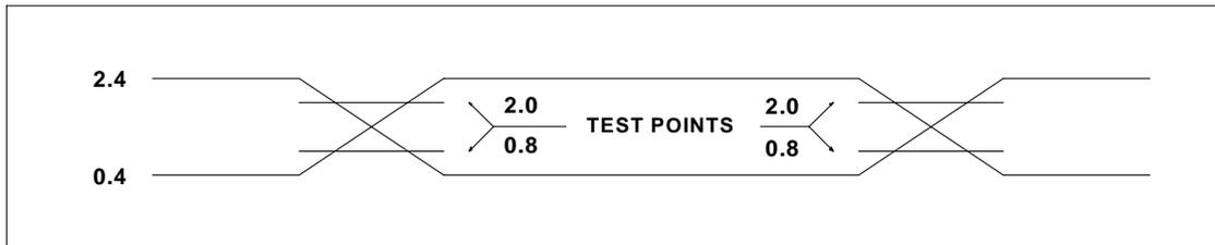
AC Testing : Input is driven at 2.4V for logic "1",and 0.4V for logic "0".Timing measurements are made at 2.0V for logic "1",and 0.8V for logic "0".
