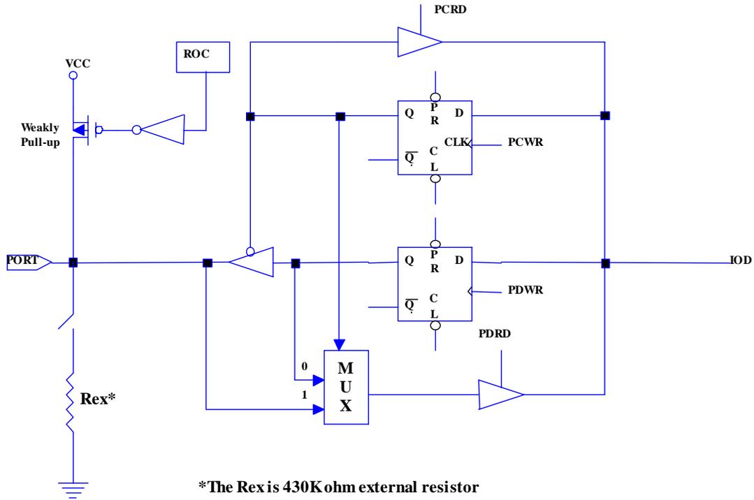
**Fig. 8 The Circuit of I/O Port with R-option(P50,P51)**
