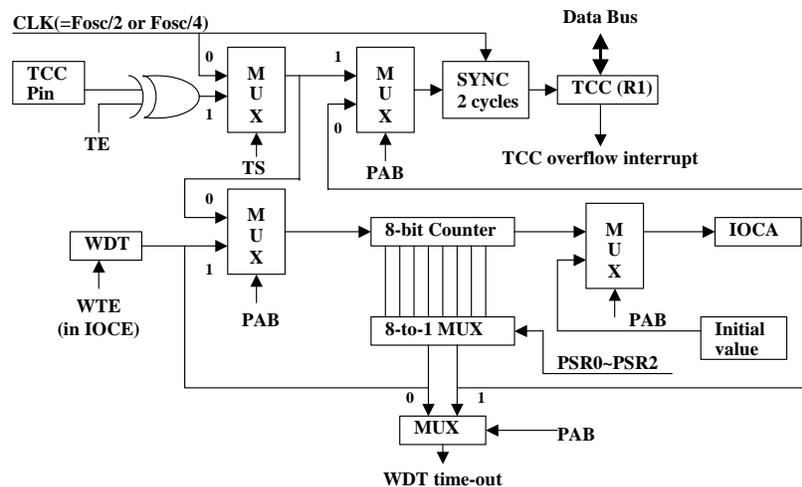
**Fig. 5 Block Diagram of TCC and WDT**
