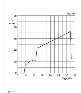
Fig.26 Quiescent current as a function of supply voltage.
