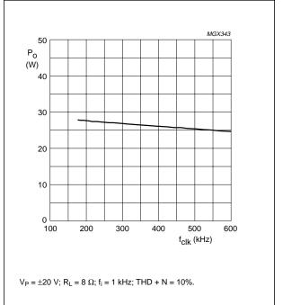
Fig.35 Output power as a function of clock frequency.
