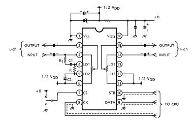
(Note) • L-ch circuit is loudness operation, R-ch circuit is without loudness.  $R_1 = 8.2k\Omega$ , C1 = 1500pF, C2 = 0.1 $\mu$ F
