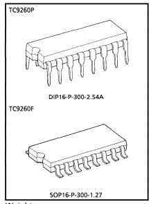
Weight DIP16-P-300-2.54A:1.0g(Typ.) SOP16-P-300-1.27 :0.16g(Typ.)
