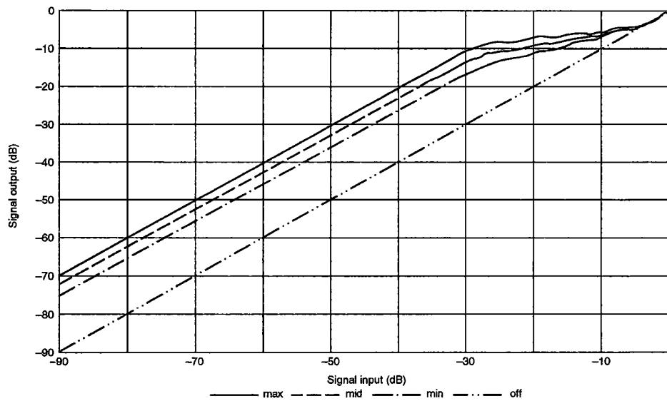
**Input/output gain characteristics**
