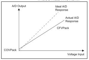
In-circuit calibration of the voltage is done at the time of manufacture to obtain absolute accuracy in addition to high resolution. Accuracy of ±40 mV at zero current and ±80 mV during charge or discharge is possible. Individual cell voltage measurements can be accurate to within ±40 mV.
