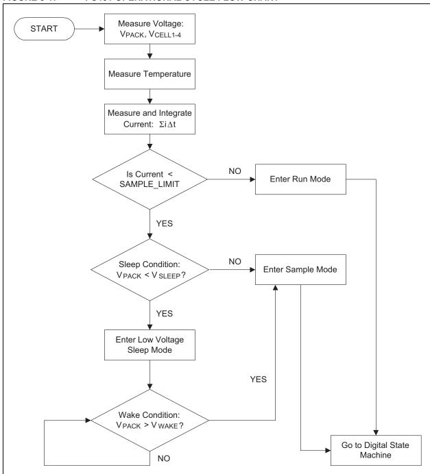
FIGURE 3-1: PS401 OPERATIONAL CYCLE FLOW CHART
