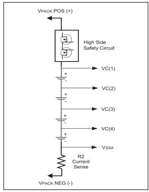
**CFVPack** is the "Correction Factor for Pack Voltage" which compensates for any variance in the actual A/D response versus an ideal A/D response over varying voltage inputs.
