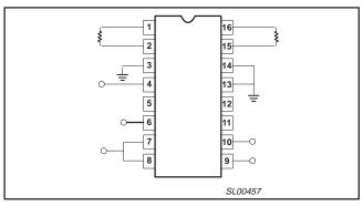
Figure 5. SA5775A Test circuit, N package
