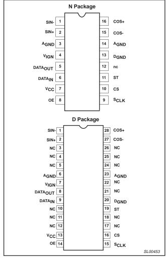
Figure 1. Pin configuration
