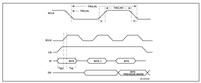
Figure 4. Serial interface timing
