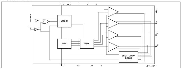
Figure 2. Block diagram, pin numbers for DIL package
