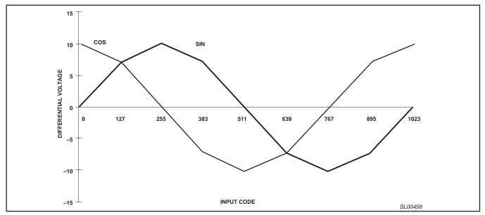
Figure 6. SA5775A output voltages (V<sub>IGN</sub> = 14 V)
