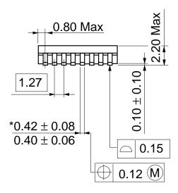
\*Dimension including the plating thickness
