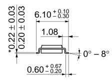
\*Dimension including the plating thickness
