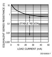
**Important:** The output capacitor must maintain its ESR within the stable region over the full operating temperature range of the application to assure stability.
