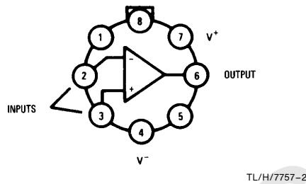
Note: Pin 4 connected to case.
