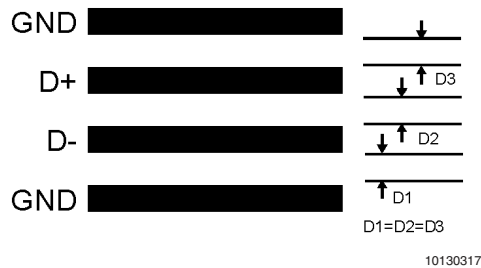
FIGURE 15. Ideal Diode Trace Layout
