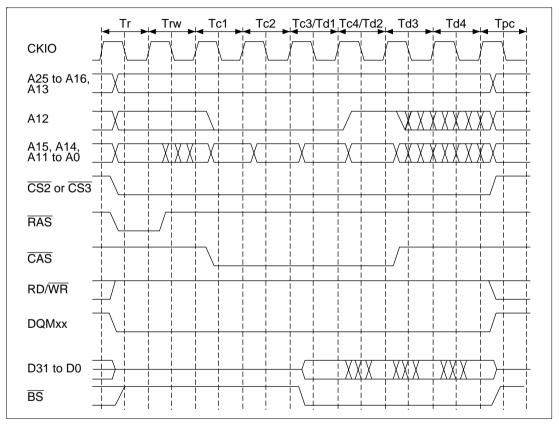
Figure 10.25 Synchronous DRAM Burst Read Wait Specification Timing
