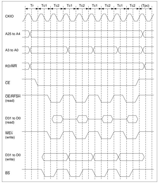
Figure 10.36 Pseudo-SRAM Static Column Mode
