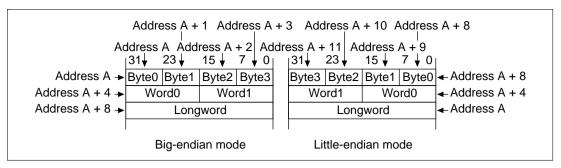
Figure 2.7 Byte, Word, and Longword Alignment
