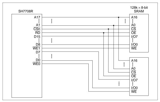
Figure 10.8 Example of 16-Bit Data Width SRAM Connection
