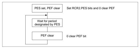
Figure 12.7 Using the Periodic Interrupt Function
