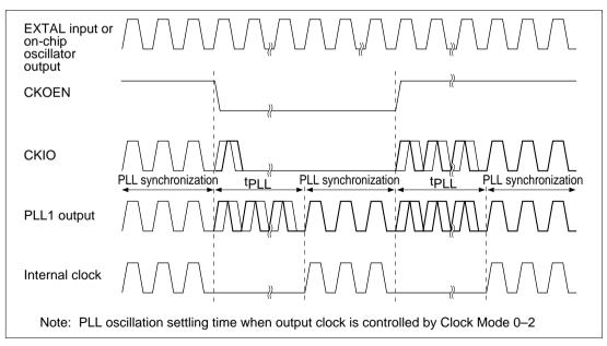
Figure 16.10 PLL Synchronization Settling Time in Case of CKOEN Bit Manipulation
