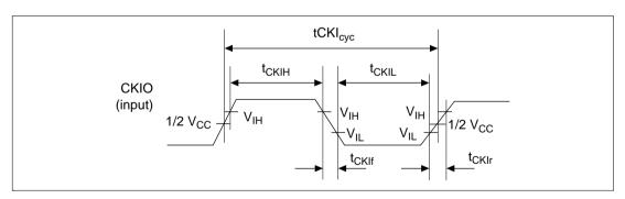
Figure 16.2 CKIO Clock Input Timing
