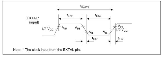
Figure 17.1 EXTAL Clock Input Timing
