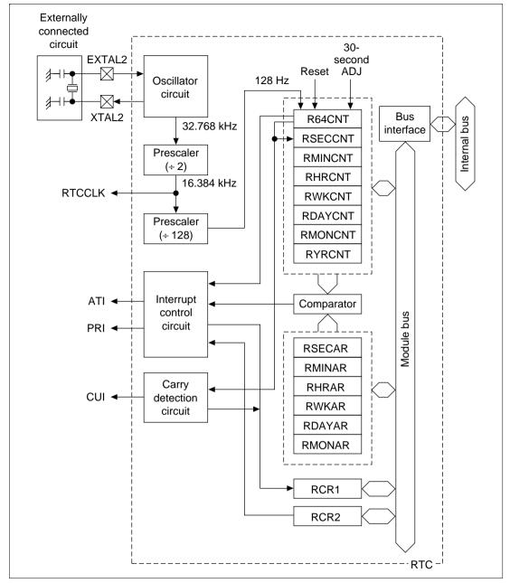
Figure 12.1 RTC Block Diagram
