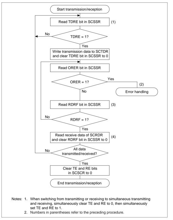
Figure 13.20 Sample Flowchart for Serial Transmitting
