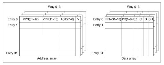
Figure 3.4 Overall Configuration of the TLB
