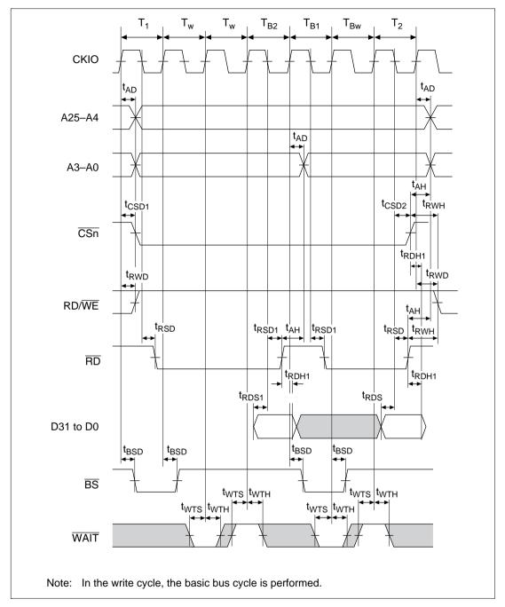
Figure 16.22 Burst ROM Bus Cycle (External Wait Input)
