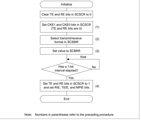
Figure 13.4 Sample Flowchart for SCI Initialization
