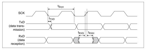
Figure 16.63 Synchronous Mode SCI Input/Output Timing
