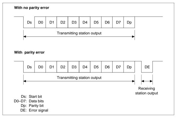
Figure 14.3 Data Format for Smart Card Interface
