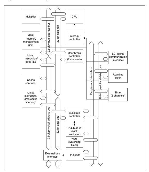
Figure 1.1 SH7708 Series Block Diagram
