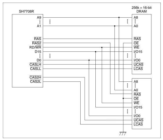
Figure 10.14 Example of DRAM Connection (16-Bit Data Width)
