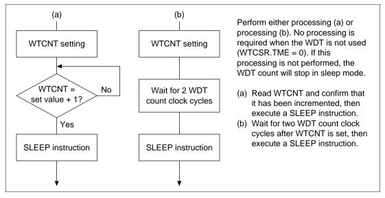
Figure 9.6 To Operate the WDT in Sleep Mode
