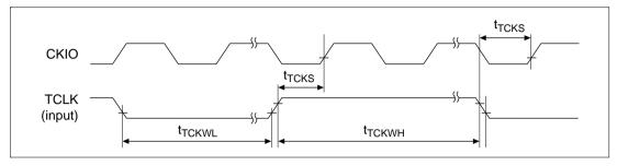
Figure 16.60 TCLK Input Timing (2)
