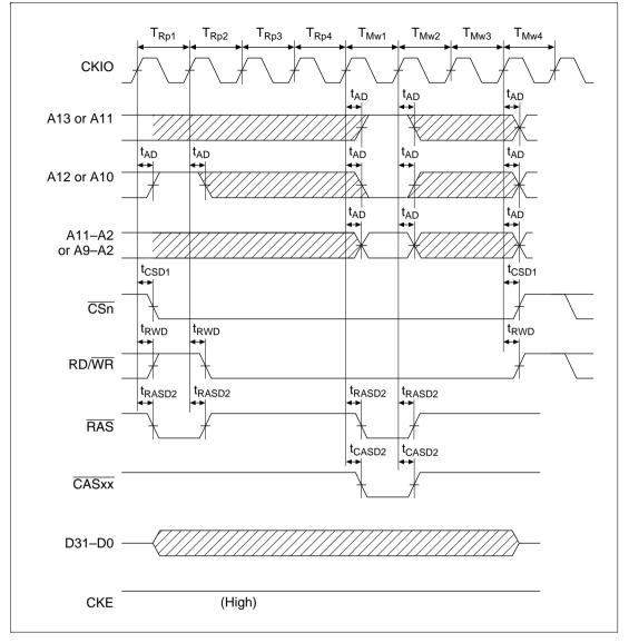
Figure 17.44 Synchronous DRAM Mode Register Write Cycle
