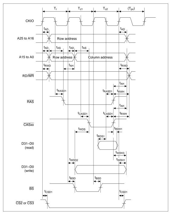
Figure 16.23 DRAM Bus Cycle (RCD = 0, AnW = 1, TPC = 0)
