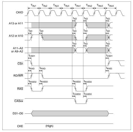
Figure 16.44 Synchronous DRAM Mode Register Write Cycle
