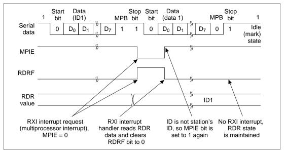
Figure 13.13 (a) Example of SCI Receive Operation: Own ID Does Not Match Data (8-Bit Data with Multiprocessor Bit and One Stop Bit)
