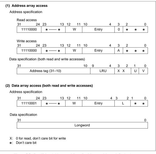
Figure 5.5 Specifying Address and Data for Memory-Mapped Cache Access
