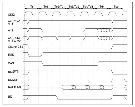
Figure 10.24 Basic Timing for Synchronous DRAM Burst Read
