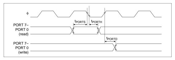
Figure 16.64 I/O Port Input/Output Timing
