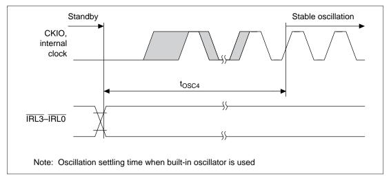
Figure 16.7 Standby Return Oscillation Settling Time (Return by IRL3-IRL0)
