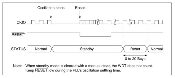
Figure 8.6 Standby to Manual Reset STATUS Output
