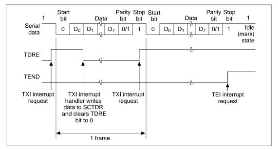
Figure 13.6 SCI Transmit Operation in Asynchronous Mode (Example: 8-Bit Data with Parity and One Stop Bit)
