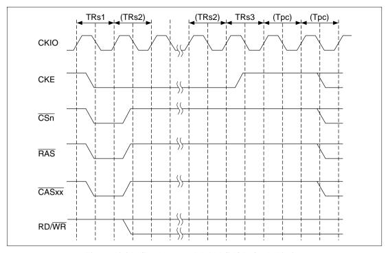
Figure 10.31 Synchronous DRAM Self-Refresh Timing
