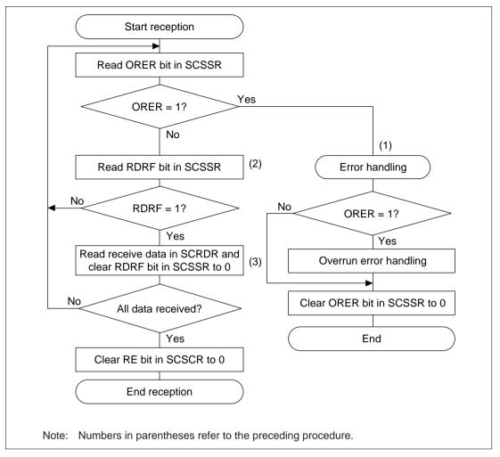
Figure 13.18 Sample Flowchart for Serial Receiving
