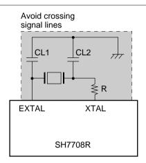
Note: The values for CL1, CL2, and the damping resistance should be determined after consultation with the crystal manufacturer.
