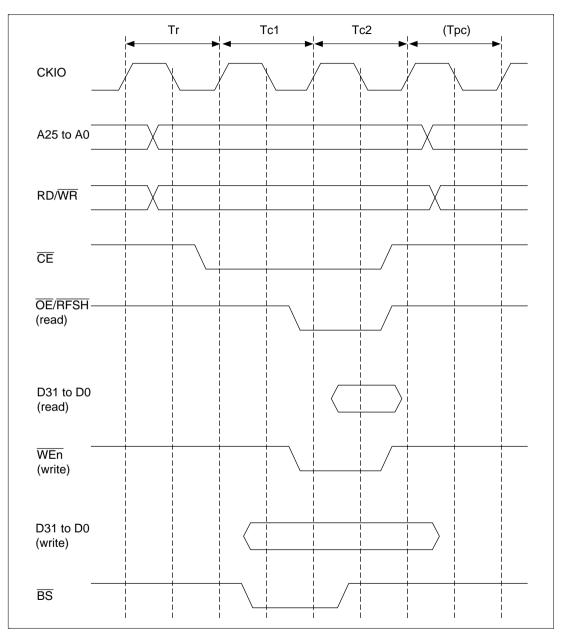
Figure 10.34 Basic Access Timing for Pseudo-SRAM
