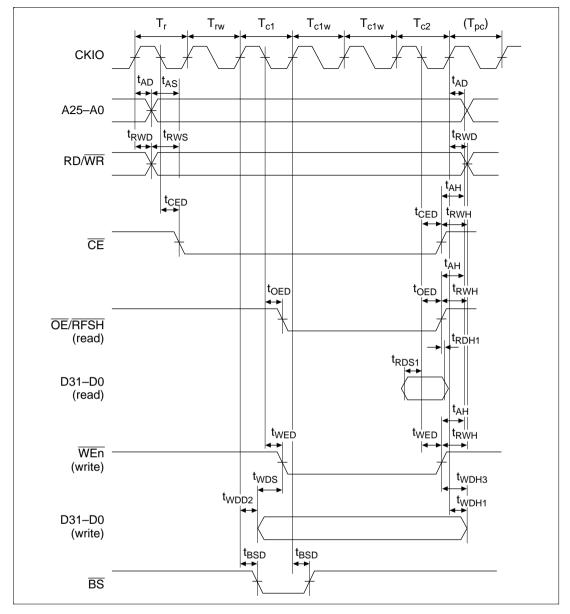
Figure 17.46 Pseudo-SRAM Read Cycle (RCD = 1, A3W = 3, TPC = 0)
