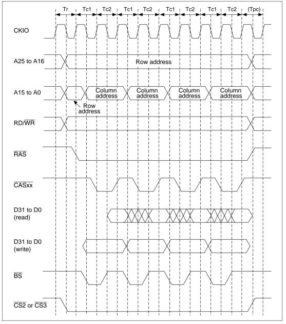
Figure 10.19 Burst Access Timing in DRAM EDO Mode
