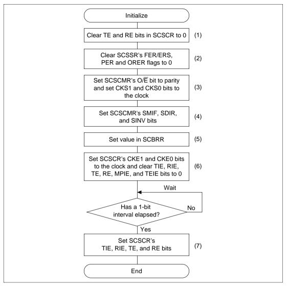
Figure 14.5 Initialization Flowchart (Example)
