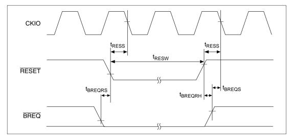
Figure 17.11 Manual Reset Input Timing
