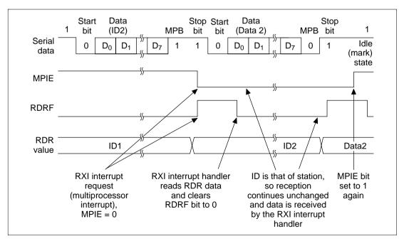
Figure 13.13 (b) Example of SCI Receive Operation: Own ID Matches Data (8-Bit Data with Multiprocessor Bit and One Stop Bit)
