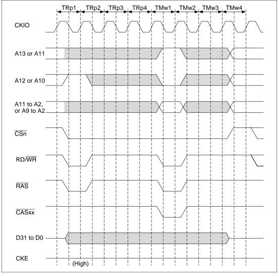
Figure 10.32 Synchronous DRAM Mode Write Timing
