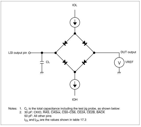
Figure 17.65 Output Load Circuit
