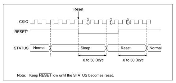
Figure 8.9 Sleep to Manual Reset STATUS Output
