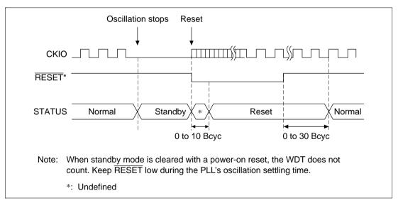
Figure 8.5 Standby to Power-On Reset STATUS Output
