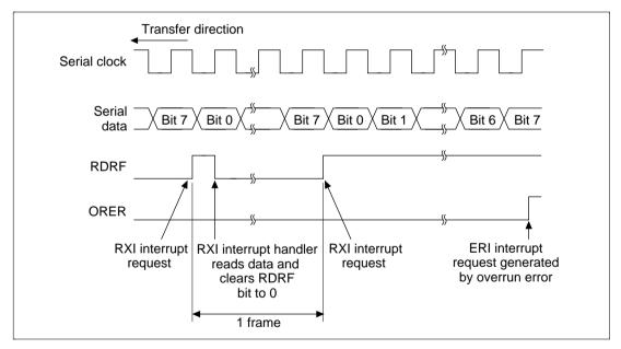
Figure 13.19 Example of SCI Receive Operation
