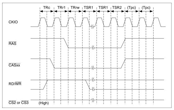
Figure 10.22 DRAM Self-Refresh Cycle Timing
