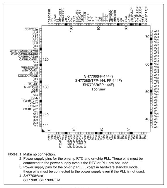
Figure 1.2 Pin Arrangement
