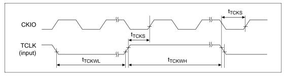
Figure 17.60 TCLK Input Timing (2)
