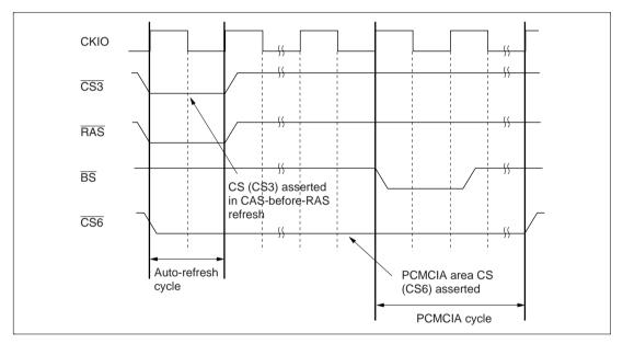
**Restrictions:** When using PCMCIA in area 6 and also using SDRAM, the area 6 CS signal (CS6) may be asserted earlier than usual, at the same time as the preceding auto-refresh cycle.
