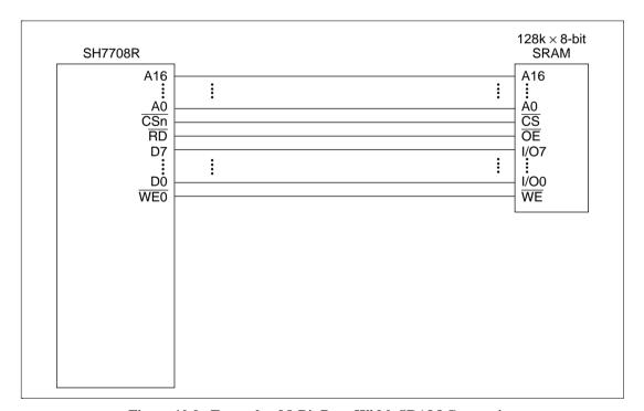
Figure 10.9 Example of 8-Bit Data Width SRAM Connection
