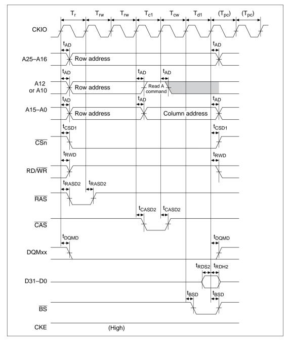
Figure 16.35 Synchronous DRAM Read Bus Cycle (RCD = 2, CAS Latency = 2, TPC = 1)
