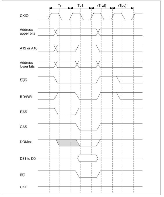
Figure 10.28 Basic Timing for Synchronous DRAM Single Write
