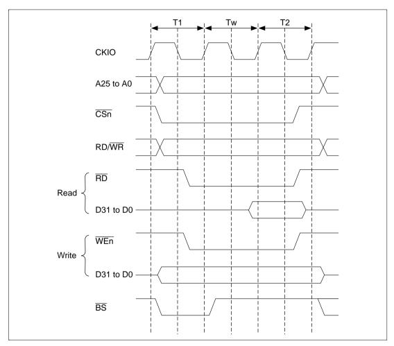
Figure 10.10 Basic Interface Wait Timing (Software Wait Only)
