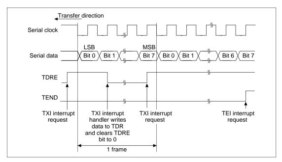
Figure 13.17 Example of SCI Transmit Operation
