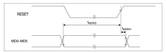
Figure 17.12 Mode Input Timing
