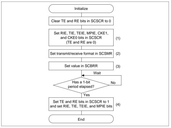
Figure 13.15 Sample Flowchart for SCI Initialization
