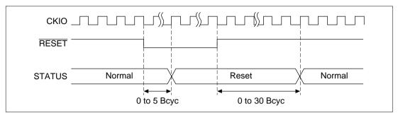
Figure 8.2 Power-On Reset (Clock Mode 3 and 4) STATUS Output
