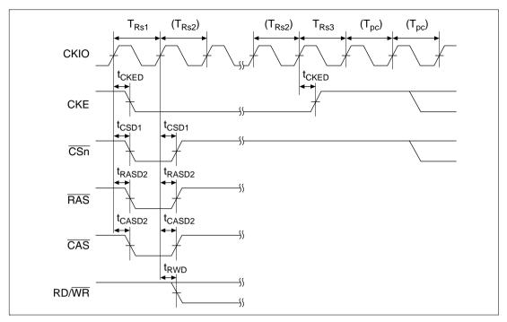
Figure 17.43 Synchronous DRAM Self-Refresh Cycle (TPC = 0)
