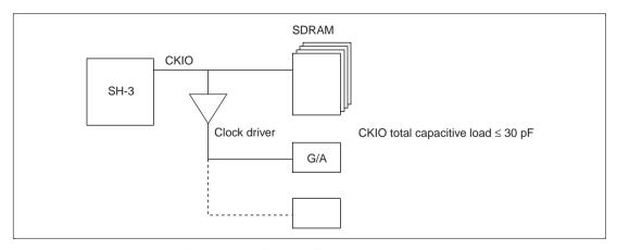
Figure 9.10 System Connection Example
