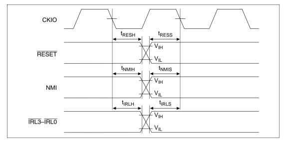
Figure 17.13 Interrupt Signal Input Timing
