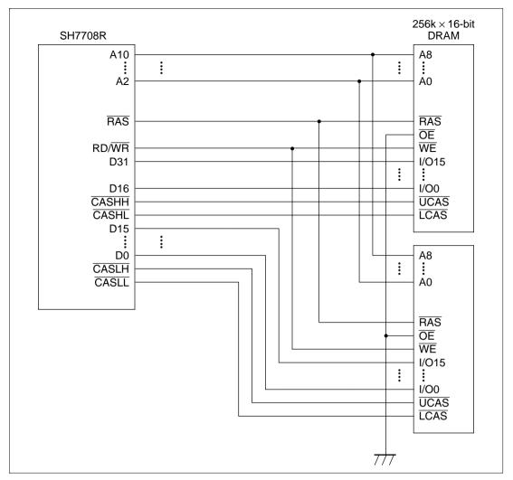
Figure 10.13 Example of DRAM Connection (32-Bit Data Width)
