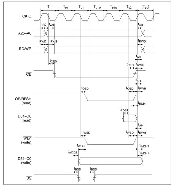
Figure 16.46 Pseudo-SRAM Read Cycle (RCD = 1, A3W = 3, TPC = 0)
