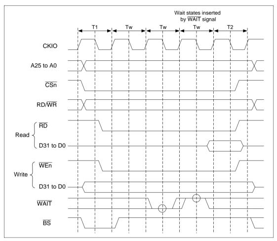
Figure 10.12 Basic Interface Wait State Timing (Wait State Insertion by  $\overline{WAIT}$  Signal, WAITSEL = 1)
