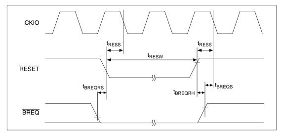
Figure 16.11 Manual Reset Input Timing
