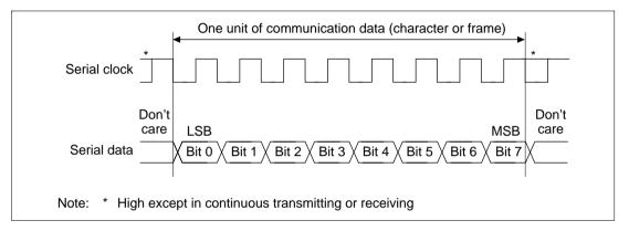
Figure 13.14 Data Format in Synchronous Communication
