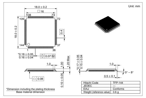
Figure D.2 Package Dimensions (TFP-144: SH7708S)
