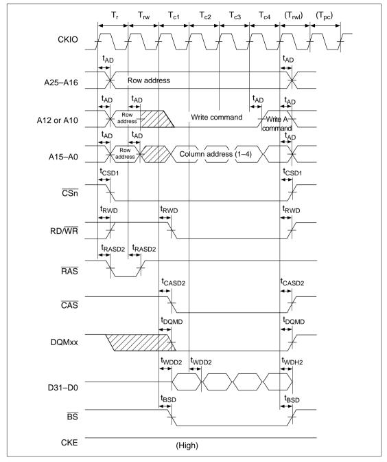
Figure 17.41 Synchronous DRAM Write Bus Cycle (Burst Mode (Single Write  $\times$  4), RCD = 1, TPC = 0, TRWL = 0)
