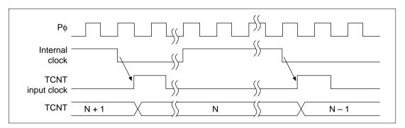
Figure 11.4 Count Timing when Internal Clock Is Operating
