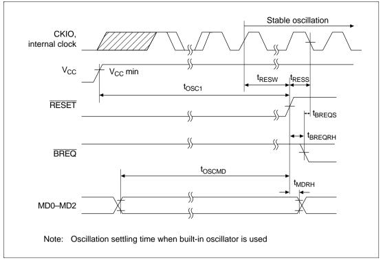
Figure 17.4 Power-On Oscillation Settling Time
