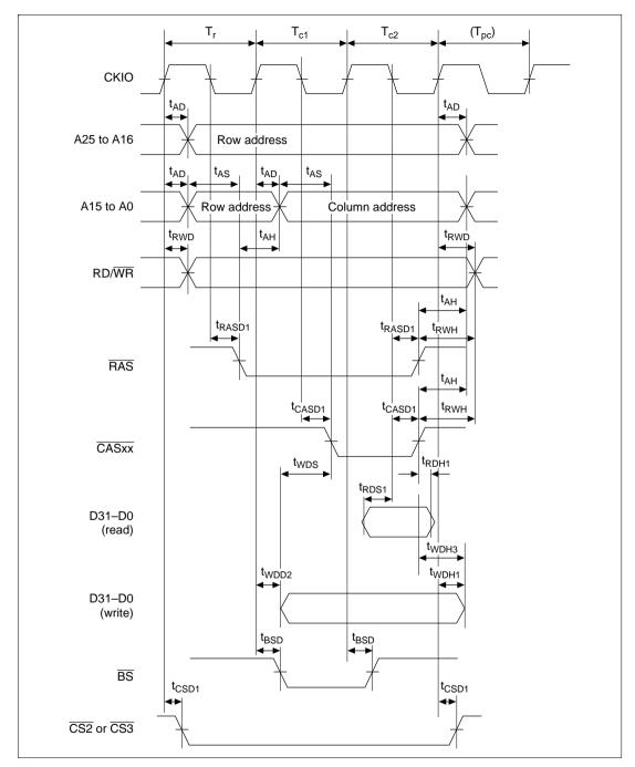
Figure 17.23 DRAM Bus Cycle (RCD = 0, AnW = 1, TPC = 0)
