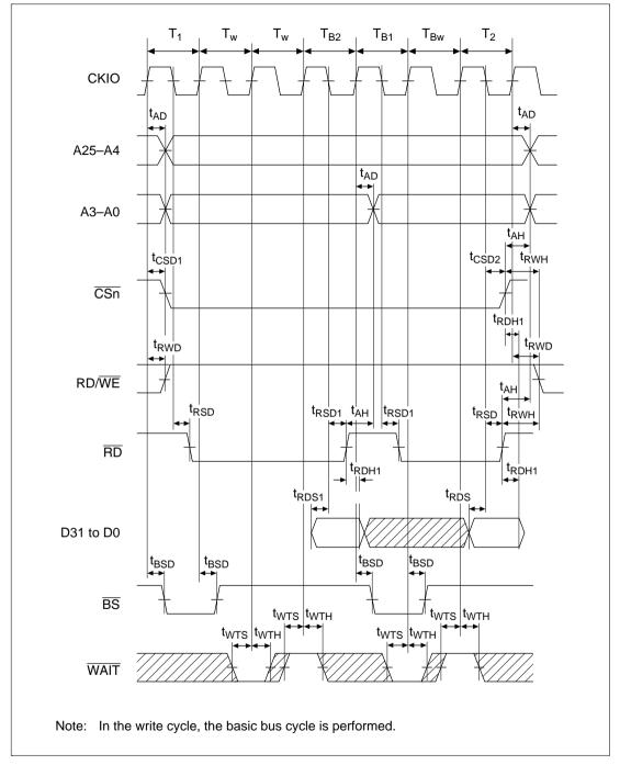
Figure 17.22 Burst ROM Bus Cycle (External Wait Input)
