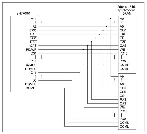
Figure 10.23 Example of Synchronous DRAM Connection
