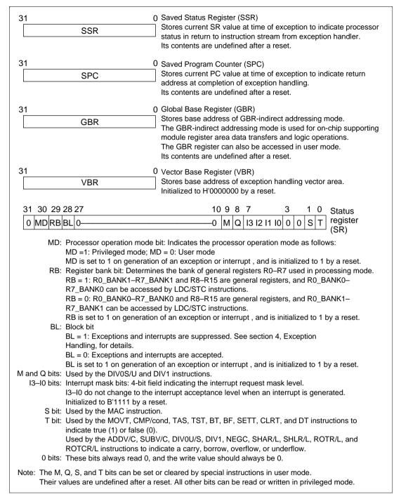
Figure 2.5 Register Set Overview, Control Registers
