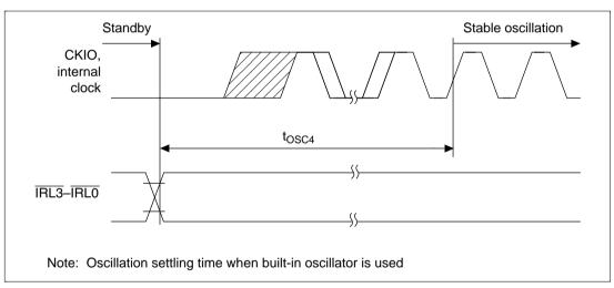
Figure 17.7 Standby Return Oscillation Settling Time (Return by IRL3-IRL0)
