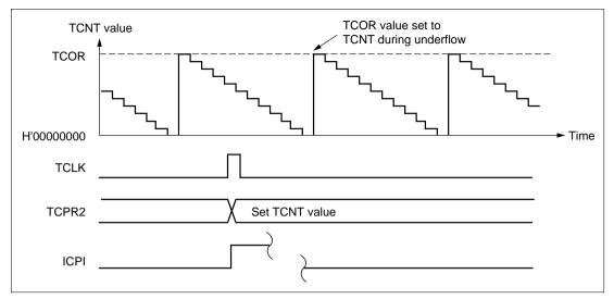
Figure 11.7 Operation Timing when Using the Input Capture Function (Using TCLK Rising Edge)
