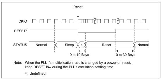
Figure 8.8 Sleep to Power-On Reset STATUS Output
