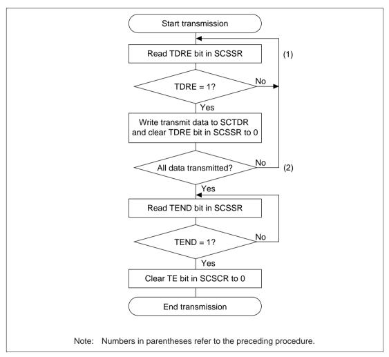
Figure 13.16 Sample Flowchart for Serial Transmitting
