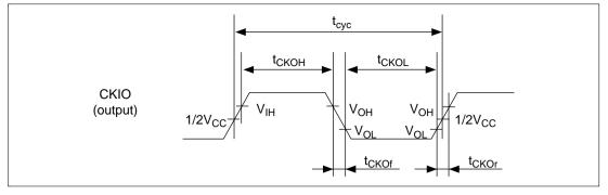
Figure 16.3 CKIO Clock Output Timing
