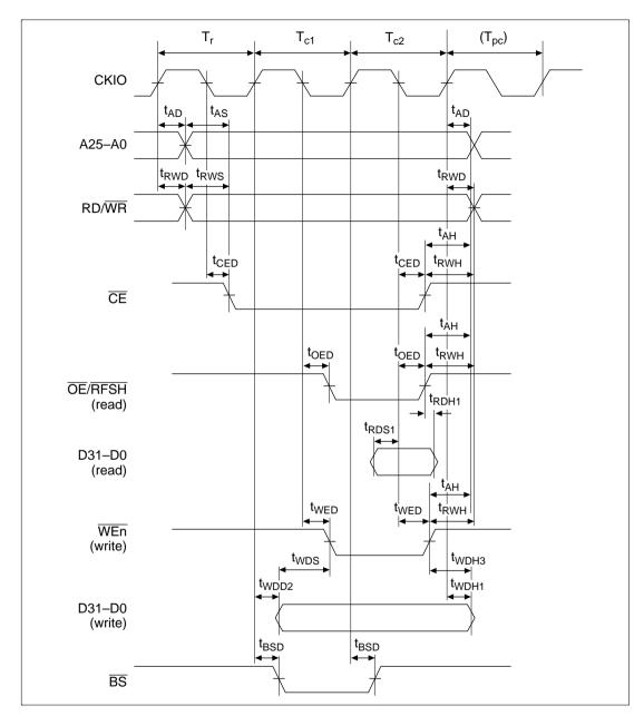
Figure 17.45 Pseudo-SRAM Bus Cycle (RCD = 0, A3W = 1, TPC = 0)
