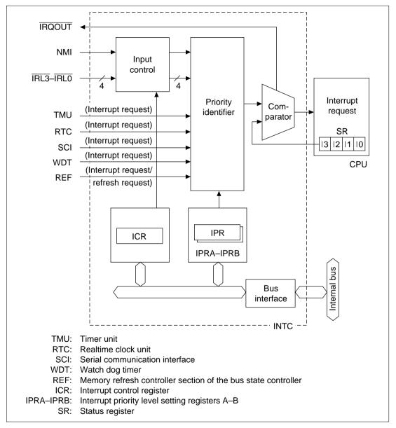
Figure 6.1 INTC Block Diagram
