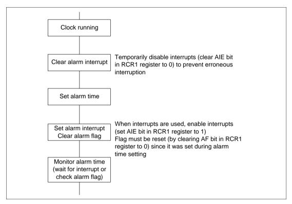
Figure 12.4 Using the Alarm Function
