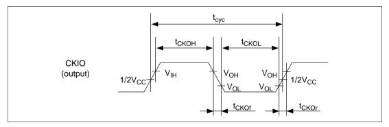
Figure 17.3 CKIO Clock Output Timing
