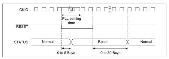
Figure 8.1 Power-On Reset (Clock Mode 0, 1, 2, and 7) STATUS Output
