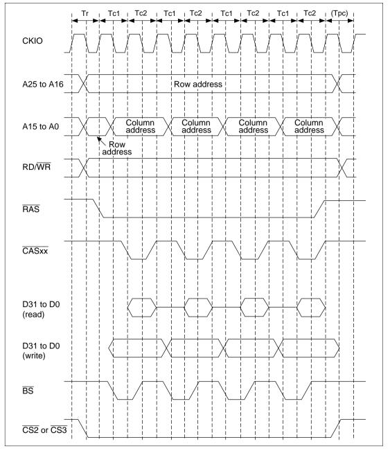
Figure 10.17 DRAM Burst Access Timing
