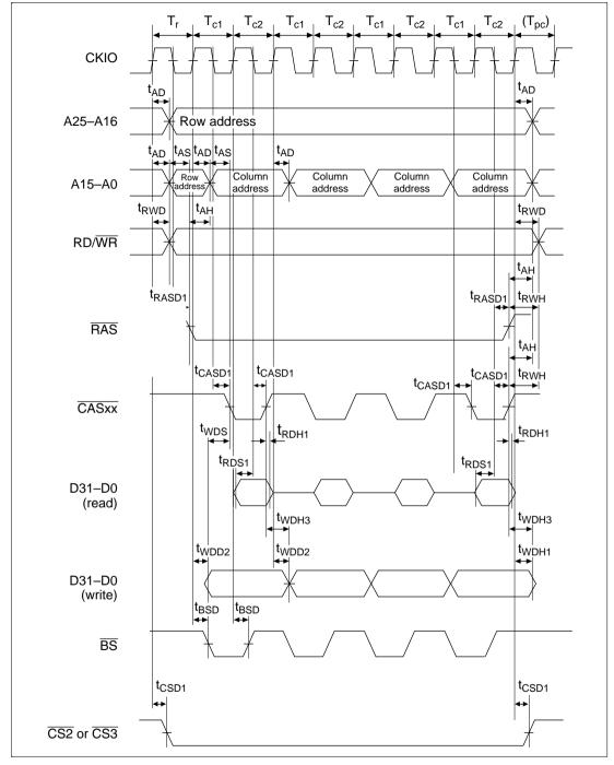
Figure 17.25 DRAM Burst Bus Cycle (RCD = 0, AnW = 1, TPC = 0)
