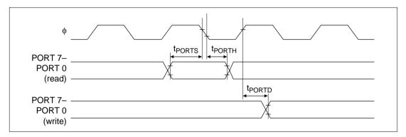
Figure 17.64 I/O Port Input/Output Timing
