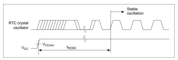
Figure 17.61 RTC Crystal Oscillator Power-On Oscillation Settling Time
