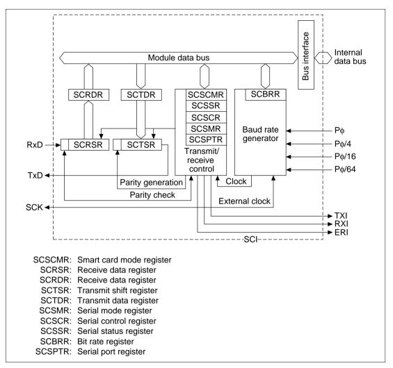
Figure 14.1 Smart Card Interface Block Diagram
