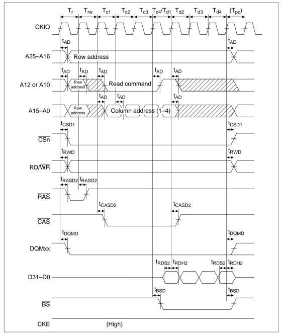
Figure 17.37 Synchronous DRAM Read Bus Cycle (Burst Read (Single Read  $\times$  4), RCD = 1, CAS Latency = 3, TPC = 0)
