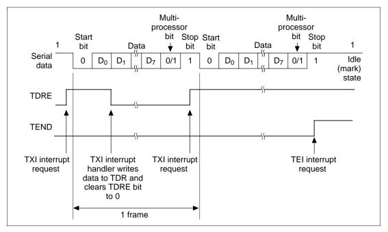
Figure 13.11 SCI Multiprocessor Transmit Operation (Example: 8-Bit Data with Multiprocessor Bit and One Stop Bit)
