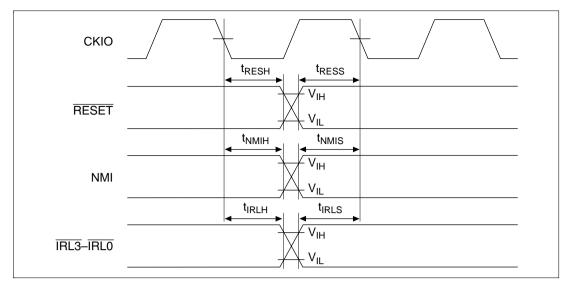
Figure 16.13 Interrupt Signal Input Timing
