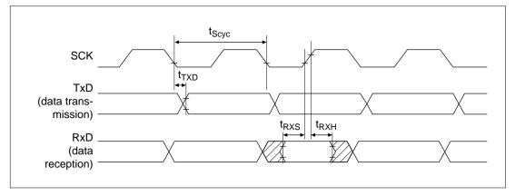
Figure 17.63 Synchronous Mode SCI Input/Output Timing
