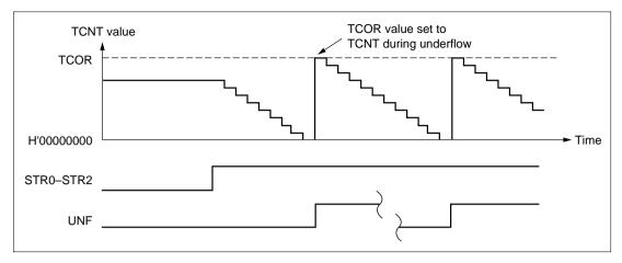
Figure 11.3 Auto-Reload Count Operation
