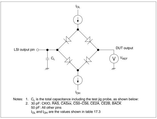
Figure 16.65 Output Load Circuit
