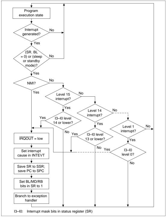
Figure 6.3 Interrupt Operation Flowchart
