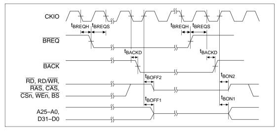
Figure 16.15 Bus Release Timing
