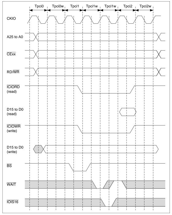
Figure 10.48 Wait Timing for PCMCIA I/O Card Interface
