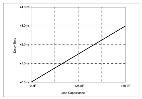
Figure C.1 Load Capacitance vs. Delay Time
