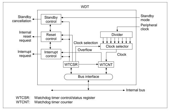
Figure 9.4 Block Diagram of the WDT
