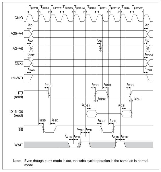
Figure 16.55 PCMCIA Memory Bus Cycle (Burst Read, TED = 1, TEH = 1, 2 Waits, Burst Pitch = 3)
