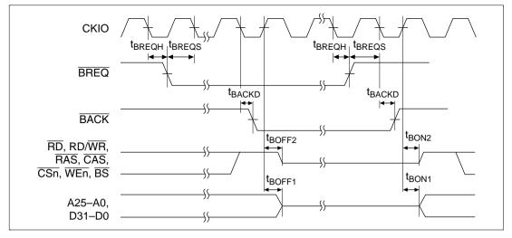
Figure 17.15 Bus Release Timing
