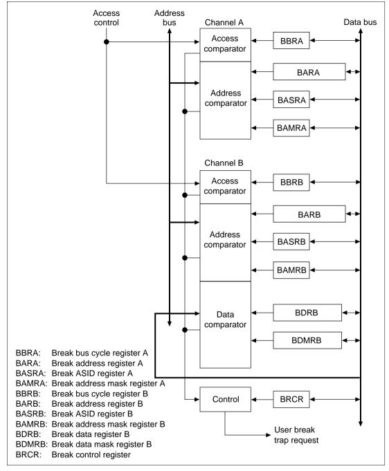
Figure 7.1 Logical Block Diagram of User Break Controller
