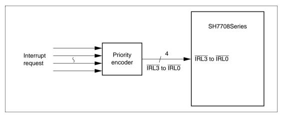
Figure 6.2 Example of IRL Interrupt Connection
