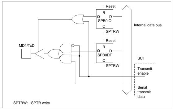
Figure 15.3 SCI I/O Port: MD1/TxD Pin
