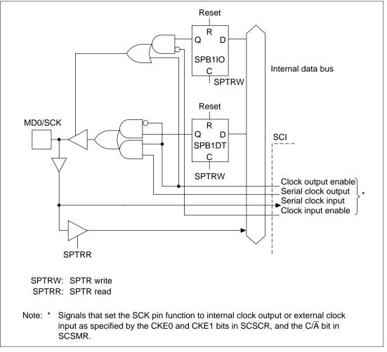
Figure 15.2 SCI I/O Port: MD0/SCK Pin
