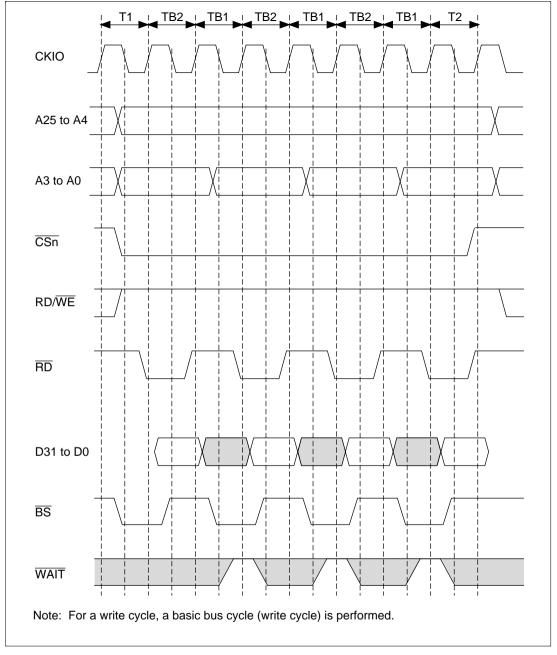
Figure 10.40 Burst ROM Basic Access Timing
