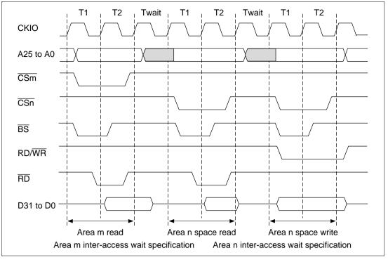
Figure 10.50 Waits between Access Cycles
