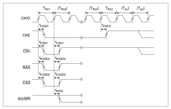
Figure 16.43 Synchronous DRAM Self-Refresh Cycle (TPC = 0)
