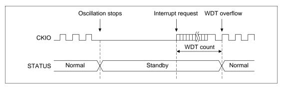
Figure 8.4 Standby to Interrupt STATUS Output
