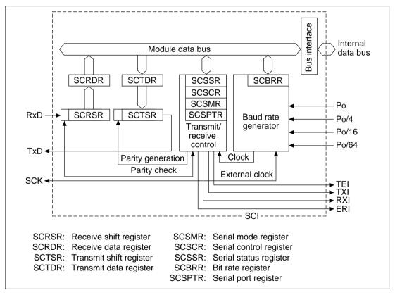
Figure 13.1 SCI Block Diagram
