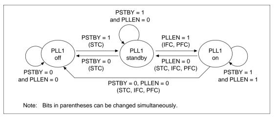
Figure 9.3 State Transitions for the PLL Standby Function
