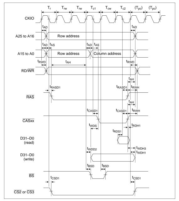
Figure 17.24 DRAM Bus Cycle (RCD = 2, AnW = 2, TPC = 1)
