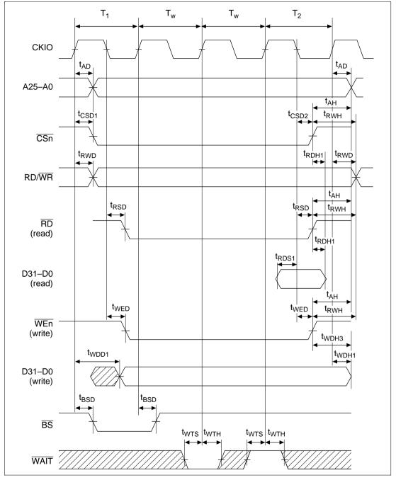
Figure 17.19 Basic Bus Cycle (External Wait)
