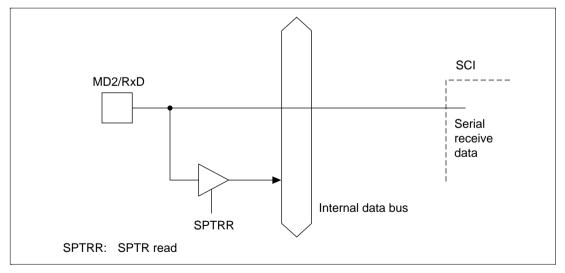
Figure 15.4 SCI I/O Port: MD2/RxD Pin
