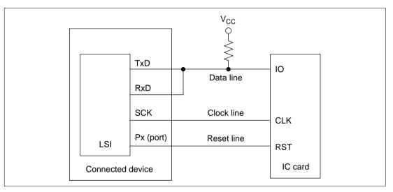
Figure 14.2 Pin Connection Diagram for the Smart Card Interface
