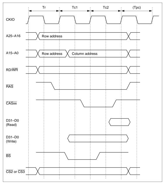
Figure 10.18 Normal Access Timing in DRAM EDO Mode
