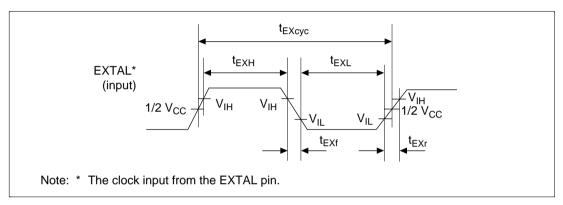
Figure 16.1 EXTAL Clock Input Timing
