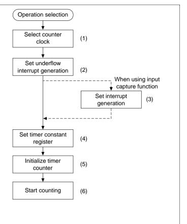
Note: When an interrupt has been generated, clear the flag in the interrupt handler that caused it. If interrupts are enabled without clearing the flag, another interrupt will be generated.
