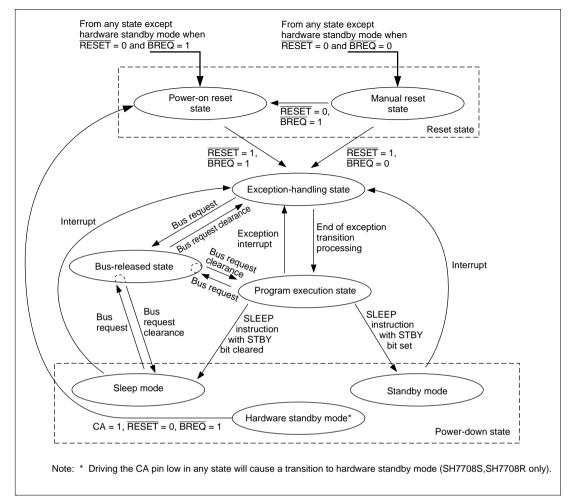
Figure 2.8 Processor State Transitions
