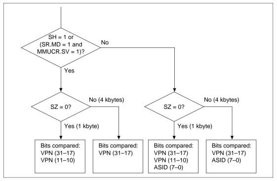
Figure 3.8 Objects of Address Comparison
