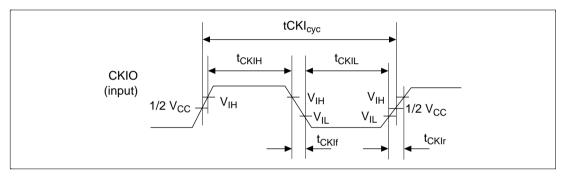
Figure 17.2 CKIO Clock Input Timing
