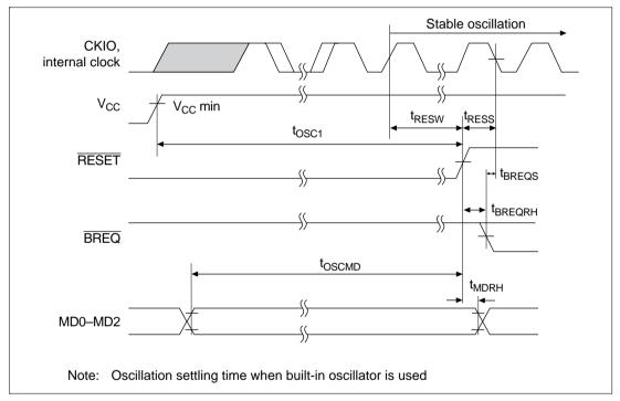
Figure 16.4 Power-On Oscillation Settling Time
