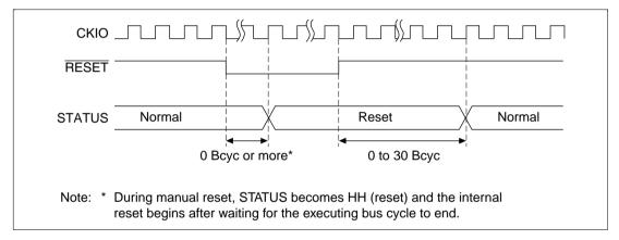
Figure 8.3 Manual Reset STATUS Output
