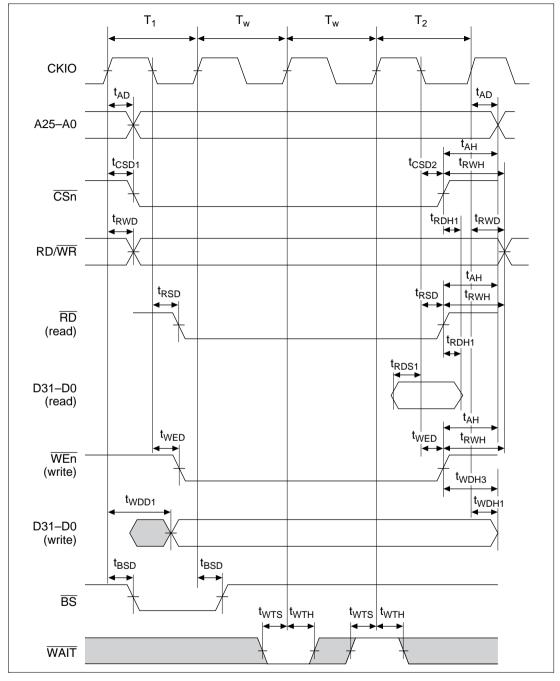
Figure 16.19 Basic Bus Cycle (External Wait)
