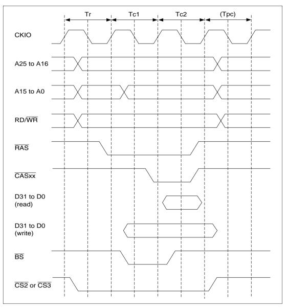
Figure 10.15 Basic Timing for DRAM Access
