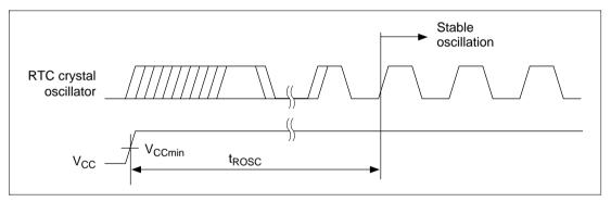
Figure 16.61 RTC Crystal Oscillator Power-On Oscillation Settling Time
