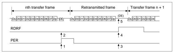
Figure 14.9 Retransmission in SCI Receive Mode
