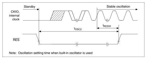
Figure 17.5 Standby Return Oscillation Settling Time (Return by RESET)
