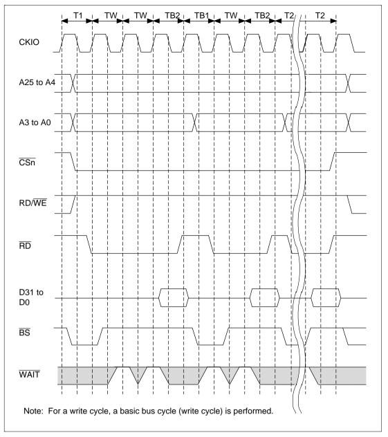
Figure 10.39 Burst ROM Wait Access Timing
