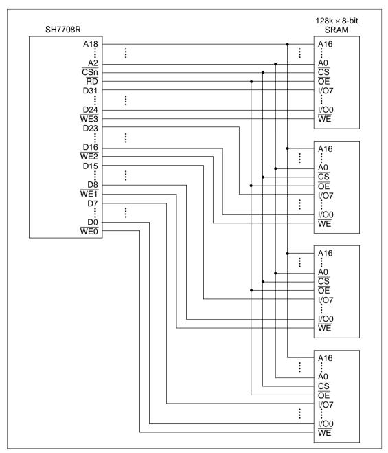
Figure 10.7 Example of 32-Bit Data Width SRAM Connection
