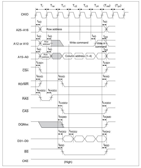
Figure 16.41 Synchronous DRAM Write Bus Cycle (Burst Mode (Single Write  $\times$  4), RCD = 1, TPC = 0, TRWL = 0)
