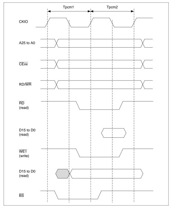
Figure 10.42 Basic Timing for PCMCIA Memory Card Interface
