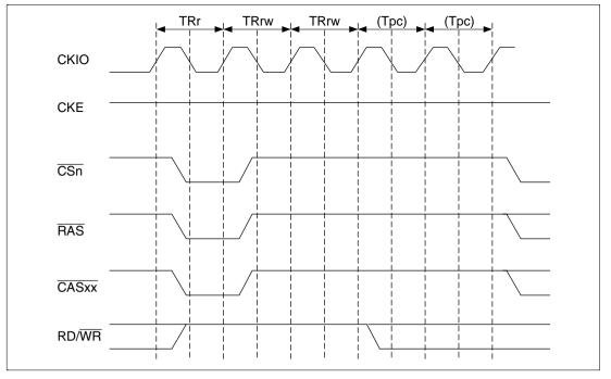
Figure 10.30 Synchronous DRAM Auto-Refresh Timing
