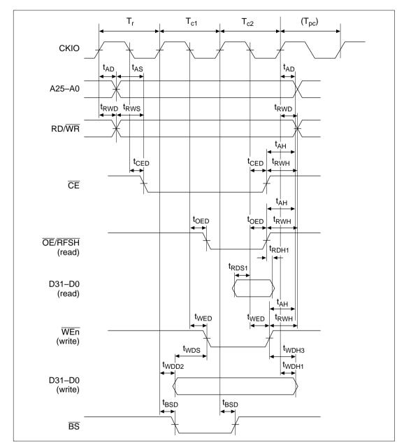
Figure 16.45 Pseudo-SRAM Bus Cycle (RCD = 0, A3W = 1, TPC = 0)
