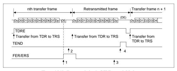
Figure 14.10 Retransmission in SCI Transmit Mode
