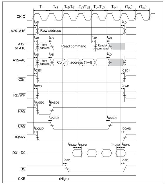
Figure 16.36 Synchronous DRAM Read Bus Cycle (Burst Read (Single Read  $\times$  4), RCD = 0, CAS Latency = 1, TPC = 1)
