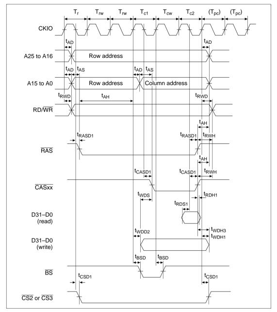
Figure 16.24 DRAM Bus Cycle (RCD = 2, AnW = 2, TPC = 1)
