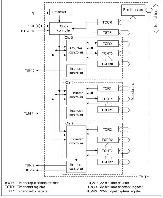
Figure 11.1 TMU Block Diagram
