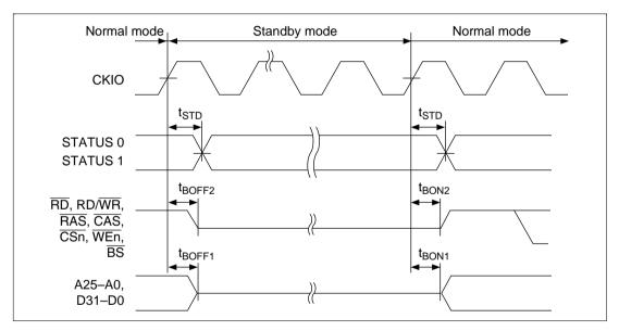
Figure 17.16 Pin Drive Timing for Standby Mode
