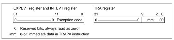
Figure 4.3 Bit Configurations of EXPEVT, INTEVT, and TRA Registers
