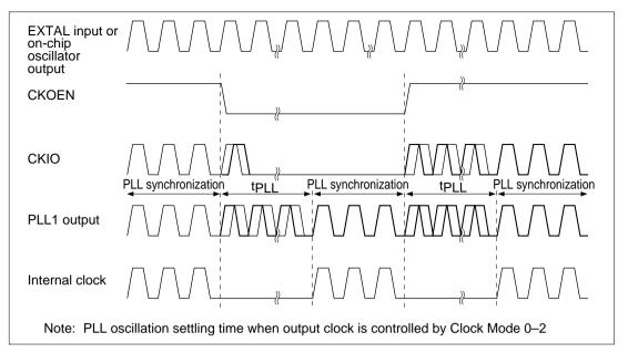
Figure 17.10 PLL Synchronization Settling Time in Case of CKOEN Bit Manipulation
