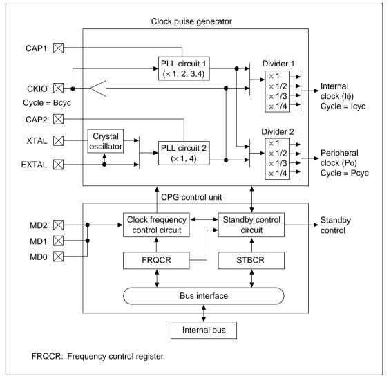
Figure 9.2 Block Diagram of Clock Pulse Generator(SH7708R)
