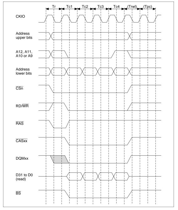
Figure 10.27 Basic Timing for Synchronous DRAM Burst Write
