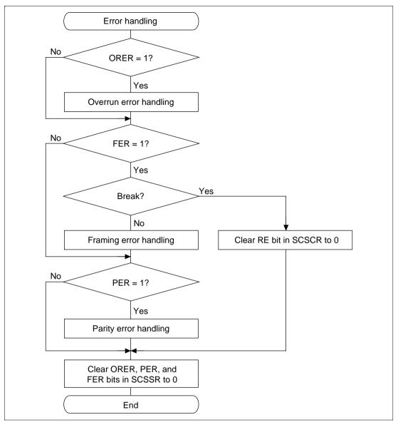
Figure 13.7 Sample Flowchart for Receiving Serial Data (cont)
