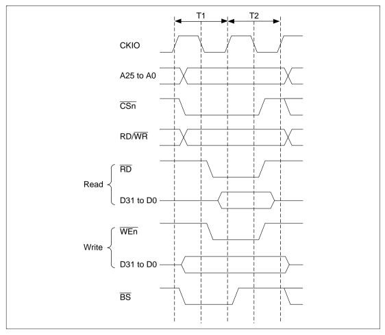
Figure 10.6 Basic Timing of Basic Interface
