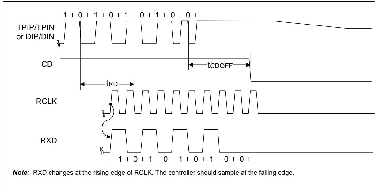
**Figure 24. Mode 2 Transmit Timing**
