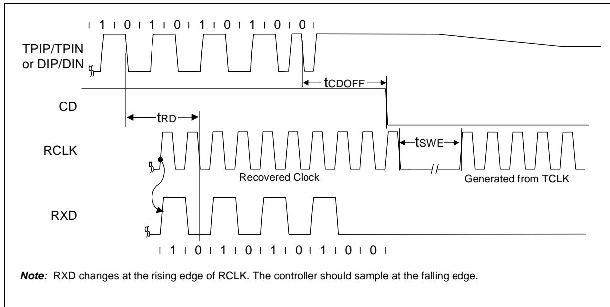
**Figure 30. Mode 3 Transmit Timing**
