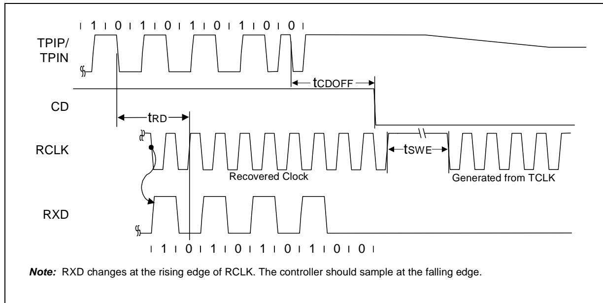
**Figure 42. Mode 5 Transmit Timing**
