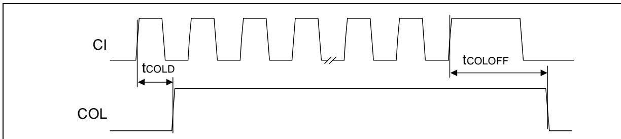
**Figure 20. Mode 1 COL/SQE Output Timing/CI Output Timing**
