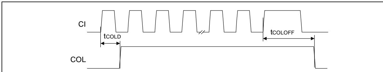
**Figure 38. Mode 4 COL/SQE Output Timing**
