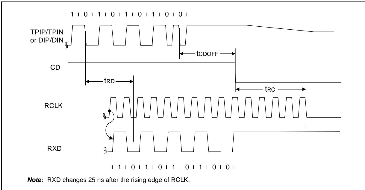
**Figure 18. Mode 1 Transmit Timing**
