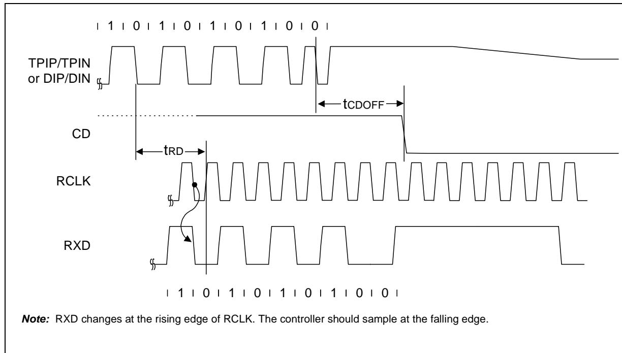
**Figure 36. Mode 4 Transmit Timing**
