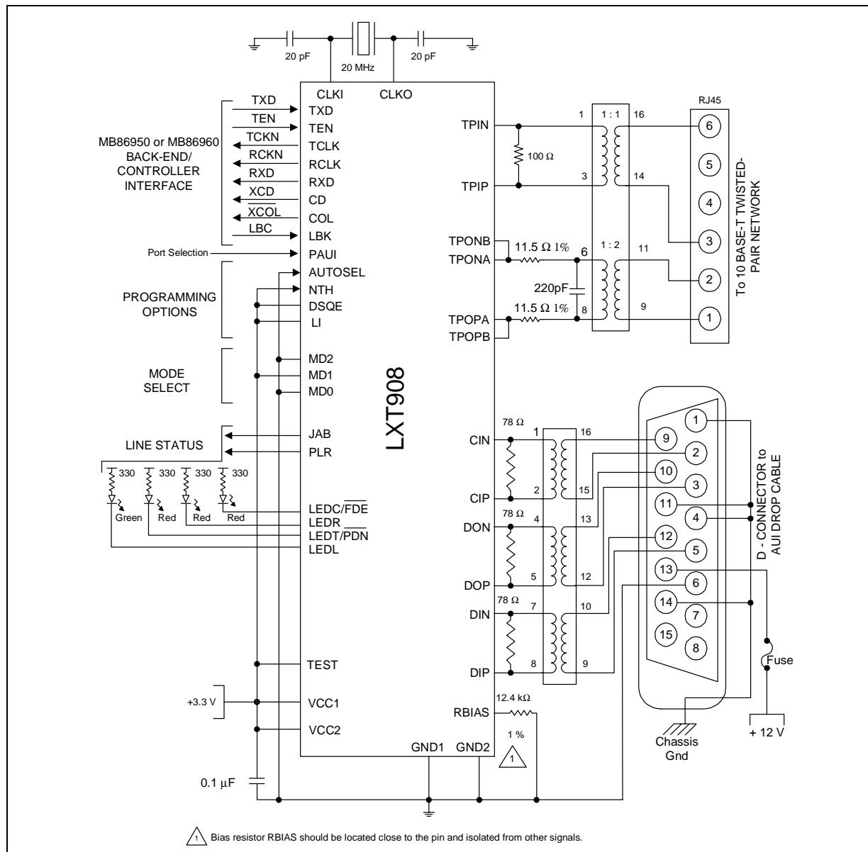
**Figure 13. Manual Port Select with Seeq 8005 Controller**
