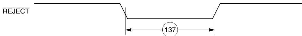
Figure 61. CAM Interface \overline{\text{REJECT}} Timing Diagram
