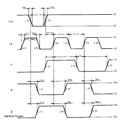
Notes) 1. Input pulse;  $t_{TLH} \le 15 \text{ ns}$ ,  $t_{THL} \le 6 \text{ ns}$ , PRR = 1 MHz and: for  $f_{max}$ ,  $t_{TLH} = t_{THL} \le 2.5 \text{ ns}$ .
