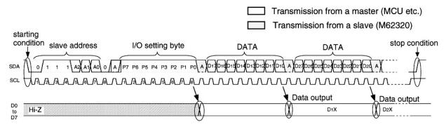
In a case of a data conversion from parallel to serial.
