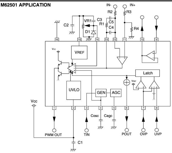
C1,C2 Stabilization capacitors of Vcc and VREF.
