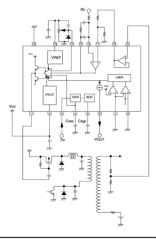
PWM IC for the synchronized deflection system control
