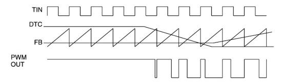
•PWM OUT ON Duty is fixed in the voltage of higher one between DTC terminal and FB terminal voltage.
