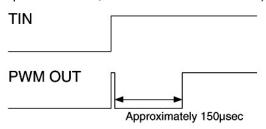
Waveform at "L" was taken from "H",and having put TIN up (PWM output is fixed in "L",too when fix TIN terminal in"L".)
