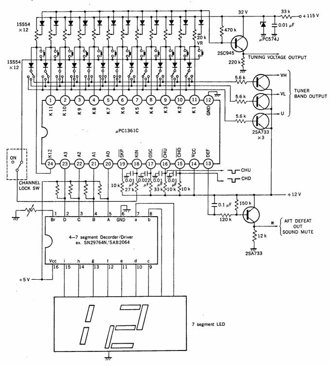
Example of TV channel selection circuit with 7 segment LED display
