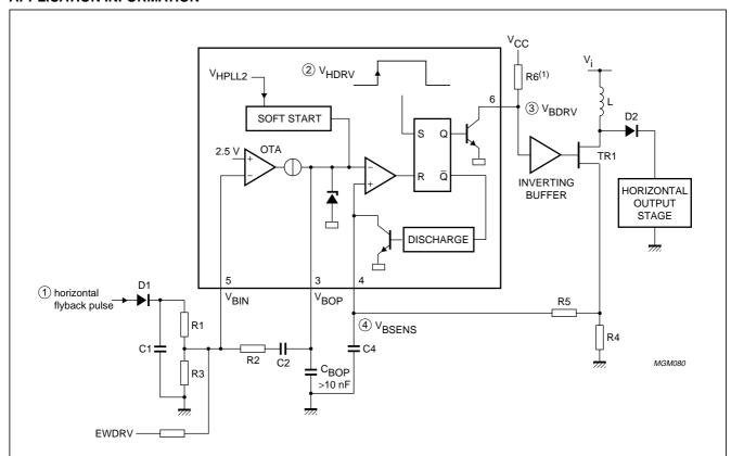
For f < 50 kHz and C2 < 47 nF calculation formulas and behaviour of the OTA are the same as for an OP. An exception is the limited output current at BOP (pin 3). See Chapter "Characteristics", subheading "B+ control section; see Figs 25 and 26".
