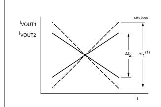
(1)  $\Delta I_1$  is the maximum amplitude setting at register VSIZE = 127, register VGAIN = 63, control bit VOVSCN = 0.
