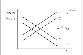
(1)  $\Delta I_1$  is the maximum amplitude setting at register VSIZE = 127 and register VGAIN = 63.
