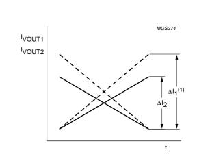
(1)  $\Delta I_1$  is the maximum amplitude setting at register VSIZE = 127, register VGAIN = 63, control bit VOVSCN = 0.
