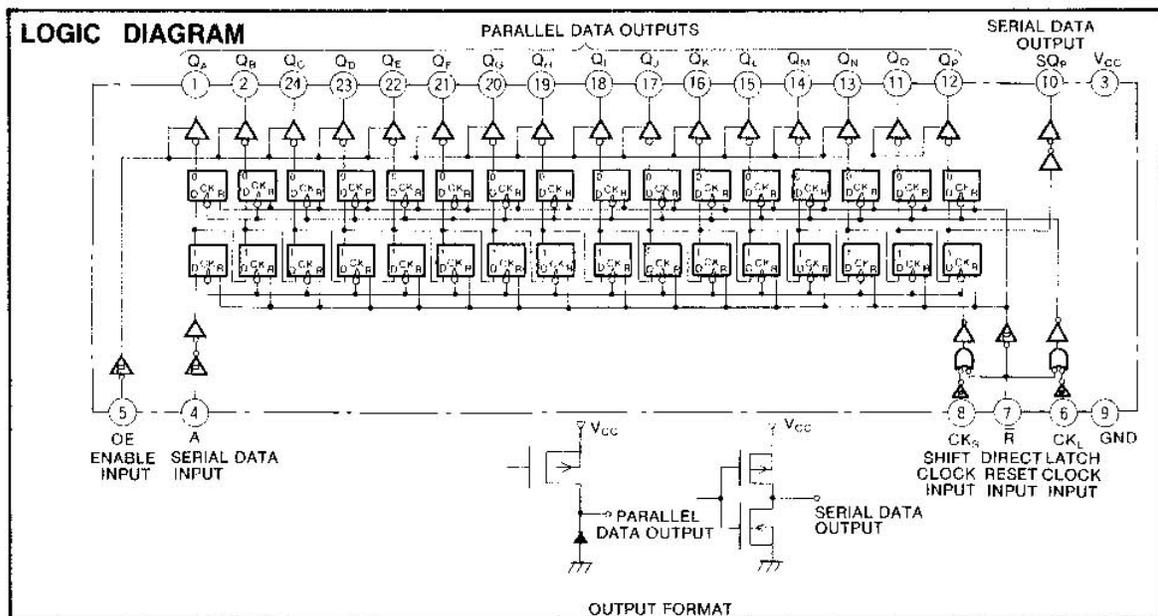
16-BIT LED DRIVER WITH SHIFT REGISTER AND LATCH
