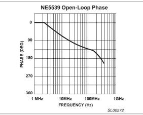
Figure 3. NE5539 Open-Loop Phase
