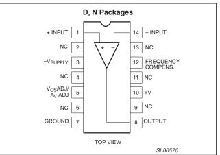
Figure 1. Pin Configuration
