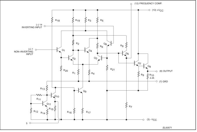
Figure 2. Equivalent Circuit
