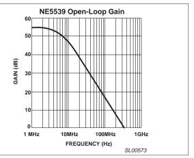
Figure 4. NE5539 Open-Loop Gain
