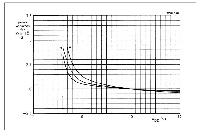
Fig.5 Typical O and  $\overline{O}$  period accuracy as a function of supply voltage; astable mode;  $T_{amb}$  = 25 °C.
