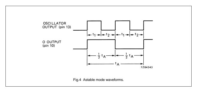
$$t_1^{} = -R_t^{}C_t^{} \ln \frac{V_{TR}^{}}{V_{DD}^{} + V_{TR}^{}}$$
