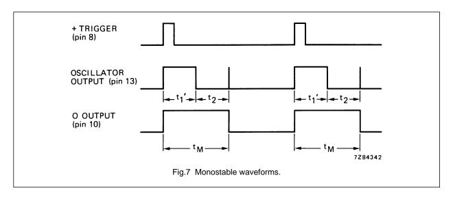
$$t_1' = -R_t C_t \ln \frac{V_{TR}}{2V_{DD}}$$
