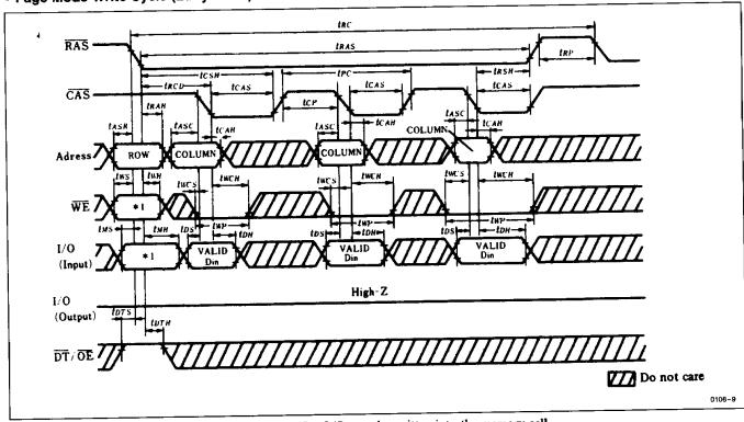
Note: \*1. When  $\overline{WE}$  is "H" level, all the data on I/O<sub>1</sub>-I/O<sub>4</sub> can be written into the memory cell.
