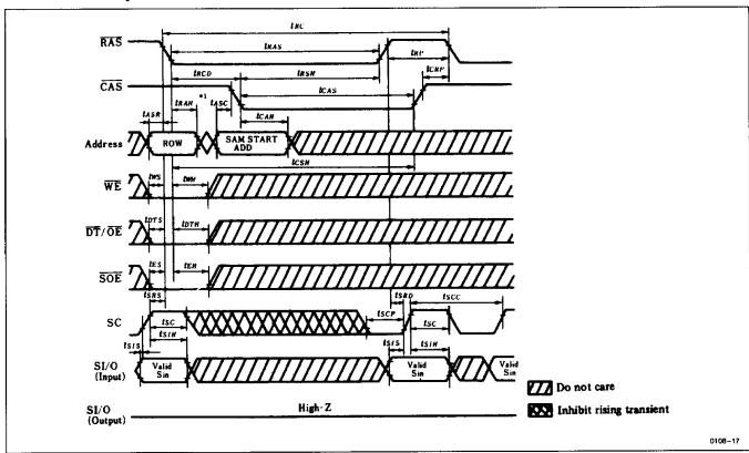
Note: \*1. CAS and SAM start address need not be supplied every cycle, only when it is desired to change to a new SAM start address.
