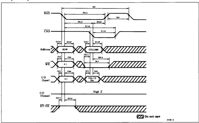
Note: \*1. When  $\overline{WE}$  is "H" level, all the data on the I/O can be written into the cell. When  $\overline{WE}$  is "L" level, the data on the I/O are not written except for when I/O is "high" at the falling edge of  $\overline{RAS}$ .
