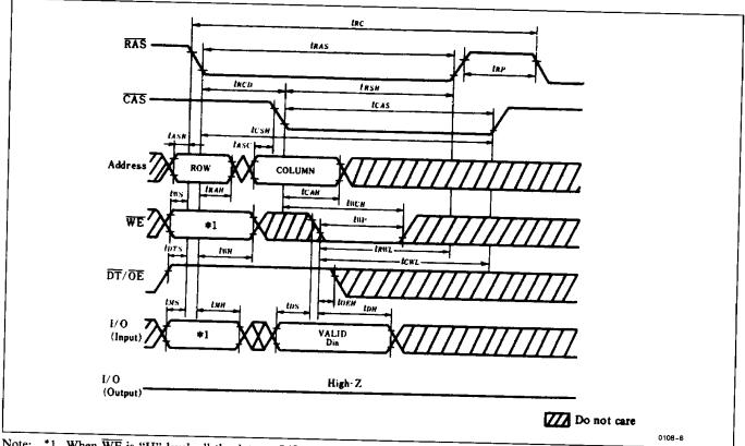
Note: \*1. When  $\overline{WE}$  is "H" level, all the data on  $I/O_1-I/O_4$  can be written into the memory cell. When  $\overline{WE}$  is "L" level, the data on I/Os are not written except for when I/O = "H" at the falling edge of  $\overline{RAS}$ .
