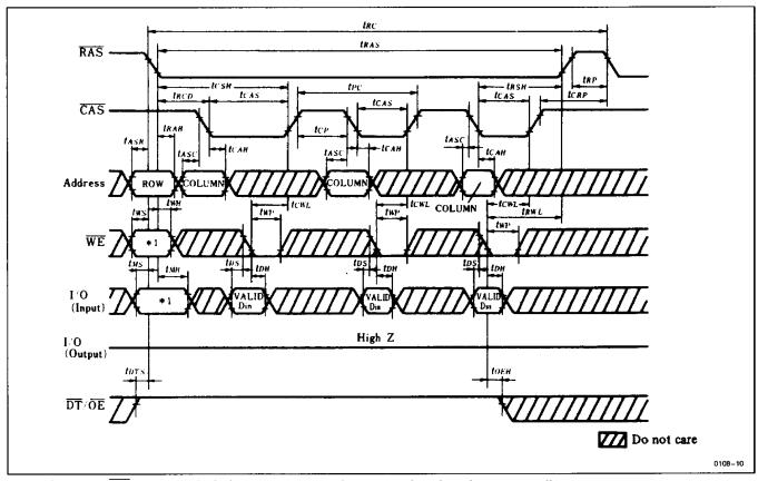
Note: \*1. When  $\overline{WE}$  is "H" level, all the data on  $I/O_1-I/O_4$  can be written into the memory cell. When  $\overline{WE}$  is "L" level, the data on  $I/O_5$  are not written except for when I/O = "H" at the falling edge of  $\overline{RAS}$ .
