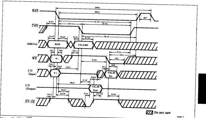
Note: \*1. When WE is "H" level, all the data on I/O<sub>1</sub>-I/O<sub>4</sub> can be written into the memory cell.
