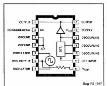
Primarily designed for use as an automotive low coolant detector, the ULN2429A monolithic bipolar integrated circuit is ideal for detecting the presence or absence of many different types of liquids in automotive, home, or industrial applications. Especially useful in harsh environments, reverse voltage protection, internal voltage regulation, temperature compensation, and high-frequency noise immunity are all incorporated in the design.
