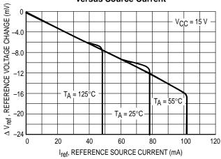
Figure 10. Reference Short Circuit Current
