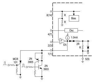
The MCR101 SCR must be selected for a holding of less than 0.5 mA at  $T_{A(min)}$ . The simple two transistor circuit can be used in place of the SCR as shown. All resistors are 10 k.
