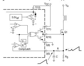
The addition of the RC filter will eliminate instability caused by the leading edge spike on the current waveform.
