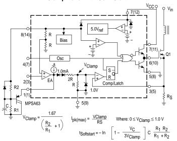
Figure 25. Current Sensing Power MOSFET
