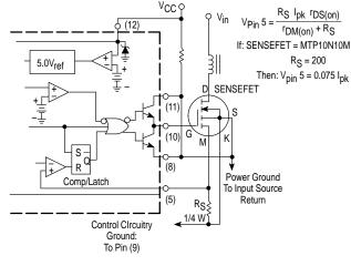
Virtually lossless current sensing can be achieved with the implementation of a SENSEFET power switch. For proper operation during over current conditions, a reduction of the  $I_{pk(max)}$  clamp level must be implemented. Refer to Figures 22 and 24.
