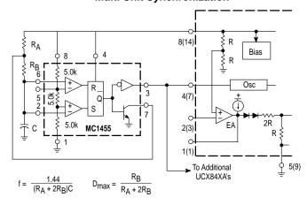
Figure 22. Adjustable Reduction of Clamp Level
