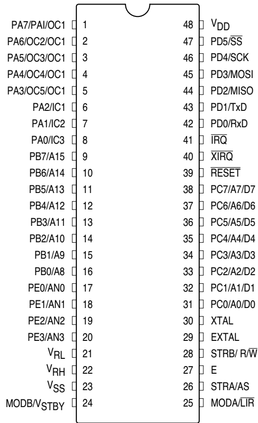
Figure 3 48-Pin DIP Pin Assignments
