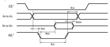
\*) The RP/RF5C01A accept  $\overline{RD}$  signals only when  $\overline{CS}$ ="L" and  $\overline{CS}$ ="L" as in the case of  $\overline{WR}$  signals. Thus, substitute  $\overline{RD}$  signals shown above, as in the case of  $\overline{WR}$  signals, with  $\overline{CS}$  ·  $\overline{RD}$  signals to be applicable to the RP/RF5C01A configuration.
