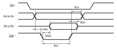
\*) The RP/RF5C01A accept  $\overline{WR}$  signals only when  $\overline{CS}$ ="L" and CS="H". Although  $\overline{CS}$  timing is not specified for the RP/RF5C01A, substitute  $\overline{WR}$  signals shown above with  $\overline{CS} \cdot \overline{WR}$  signals to be applicable to the RP/RF5C01A configuration.
