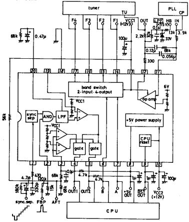
VTR application: In VTR applications without flyback pulse, connected pin 2 to  $V_{CC}$  through a resistor
