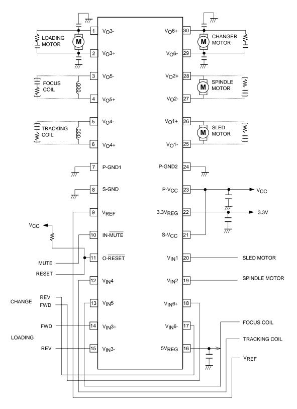
Note: When connecting a load to CH3 and CH6, set the output capacitor to  $0.56\mu$ F or more and select the capacitor according to the setting. The capacitor to be used should be less in capacity fluctuation due to temperature.
