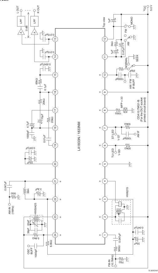
The places that differ with the LA1833 are (1) the value of the pin 8 resistor and (2) the circuits in the vicinity of pins 17 and 18. \*: Pins with the same functionality as those on the LA1832.
