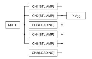
Note: • Connect both S-V<sub>CC</sub> and P-V<sub>CC</sub> to the power supply system externally. • Connect both S-GND and P-GND to the ground system externally.
