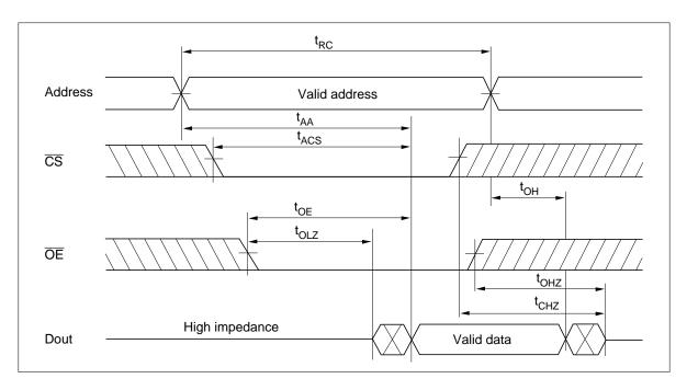
**Read Timing Waveform (1)**  $(\overline{WE} = V_{IH})$
