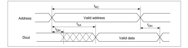
Read Timing Waveform (3)  $(\overline{WE} = V_{IH}, \overline{OE} = V_{IL})^{*3}$
