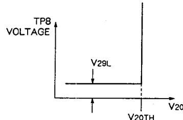
**Note13. Minimum voltage at pin 28 "V29L"**
