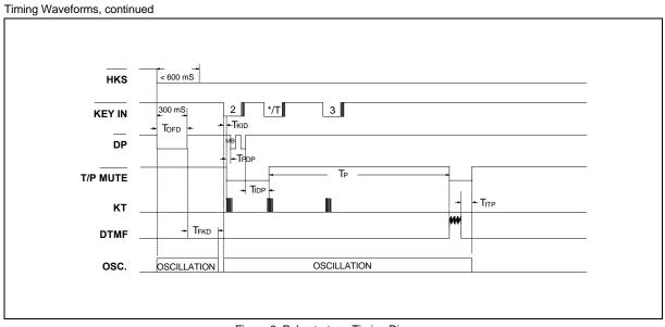
Figure 6. Pulse-to-tone Timing Diagram
