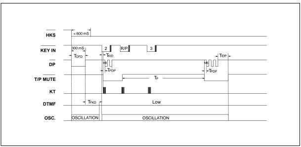
Figure 5. Pause Function Timing Diagram
