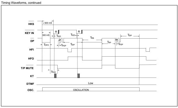
Figure 4. One-key Redial Timing Diagram (Pulse Mode)
