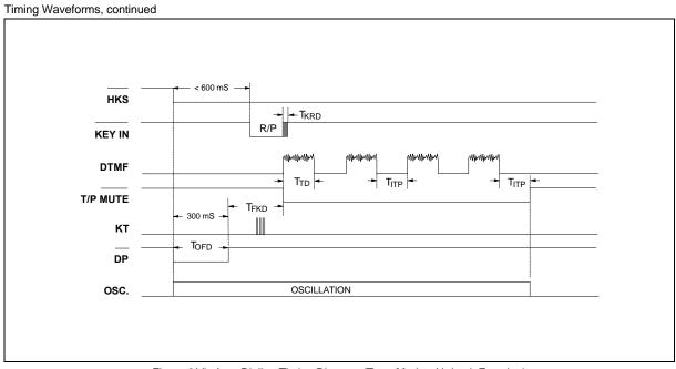
Figure 2(d). Auto Dialing Timing Diagram (Tone Mode with Lock Function)
