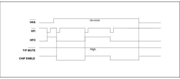
Figure 3. Handfree Dialing Timing Diagram
