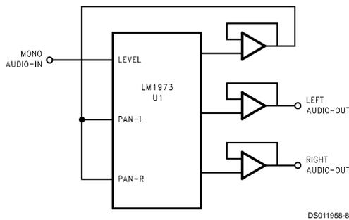
**FIGURE 6. Mono Level Control with Panning Circuit**
