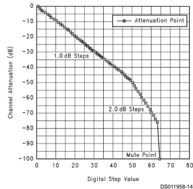
FIGURE 4. LM1973 1.0dB and 2.0dB Attenuation Step Scheme
