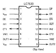
Note 1: No bonding exists on the inside of NC pin. It is recommended that the outside should be shorted to  $V_{DD}$ ,  $V_{SS}$ , etc. on the printed circuit board.
