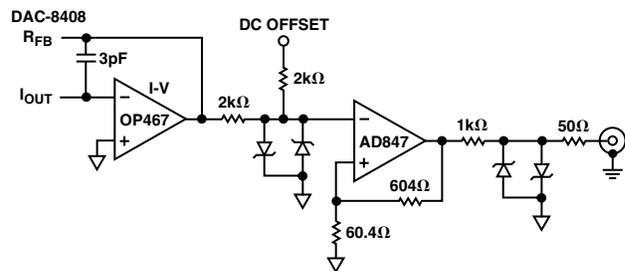
Figure 15. DAC V<sub>OUT</sub> Settling Time Circuit
