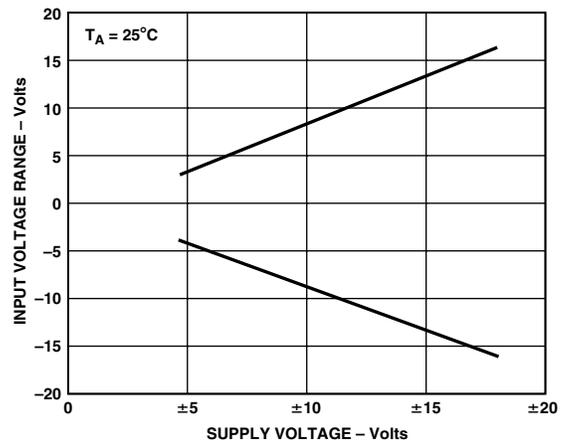
TPC 18. Input Voltage Range vs. Supply Voltage
