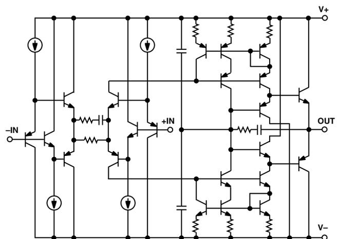
Figure 1. Simplified Schematic
