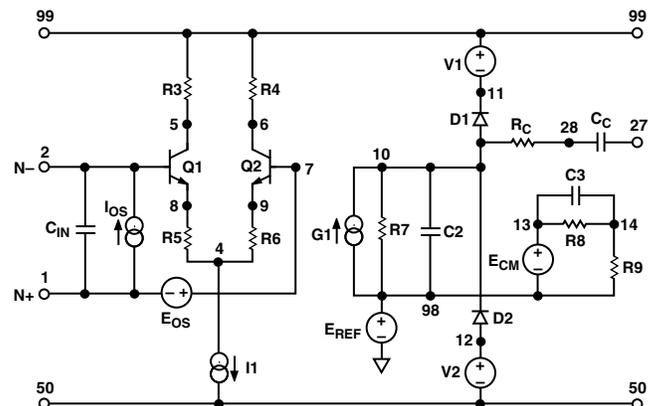
Figure 17. SPICE Macro-Model Input and Gain Stage
