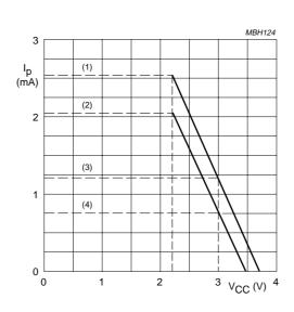
Curve (1) is valid when the receiving amplifier is not driven or when MUTE = HIGH. Curve (2) is valid when MUTE = LOW and the receiving amplifier is driven;  $V_{O(rms)} = 150 \text{ mV}$ ;  $R_L = 150 \Omega$  asymmetrical.
