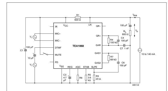
Voltage gain is defined as;  $G_v = 20 \log |V_o V_i|$ . For measuring the gain from MIC+ and MIC-, the MUTE input should be LOW or open, for measuring the DTMF input, MUTE should be HIGH. Inputs not under test should be open.
